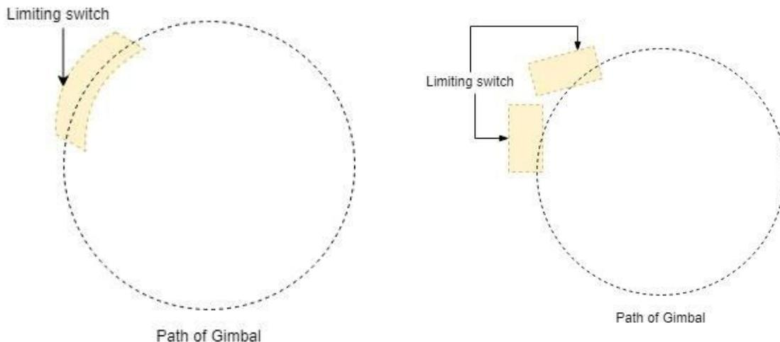
Figure 7.1.1.1 - Gimbal path and switch allocation: (a) old and (b) new location.
