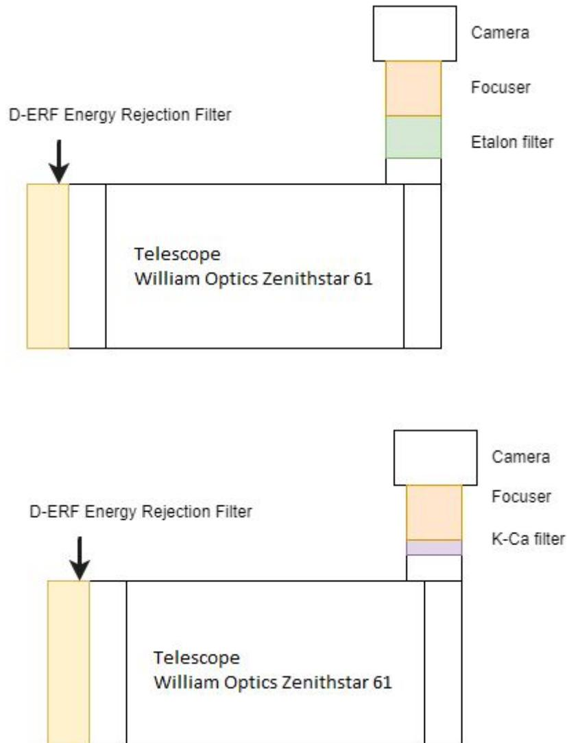
Figure 4.1.4.1 – Schematic of optical system
