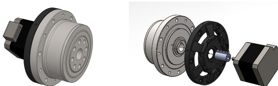
**Figure 4.3.6.2.1** - Motor, Bracket, and Harmonic Drive Assembly. The Motor Bracket was manufactured by SLM which allowed for mass saving optimizations.
