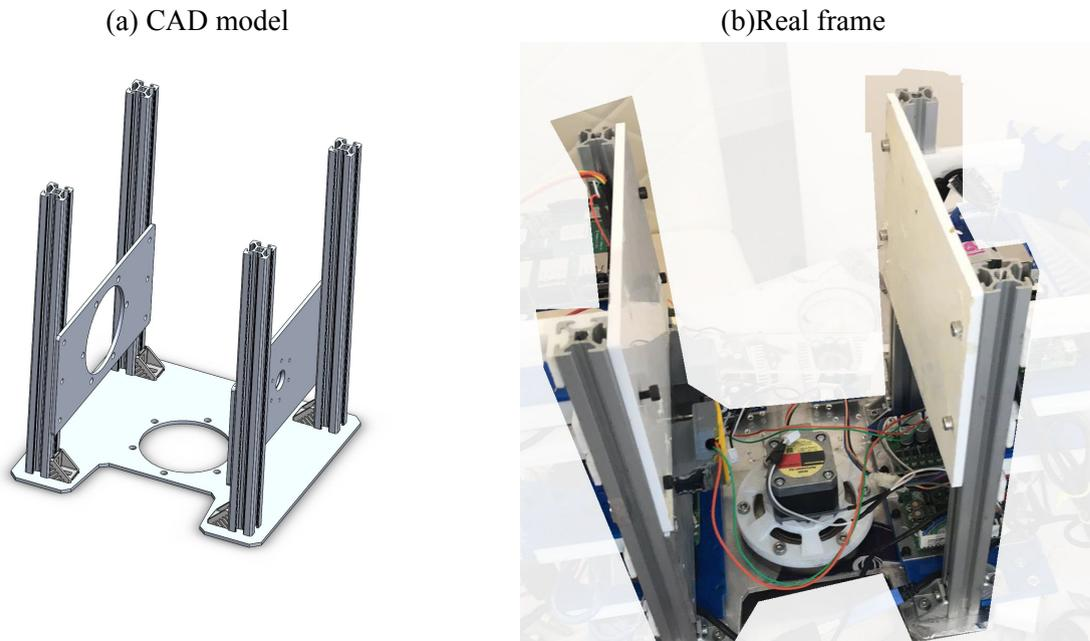
Figure 4.4.1.1 - Bosch Extrude frame with 3mm Aluminium 6010 plates.
