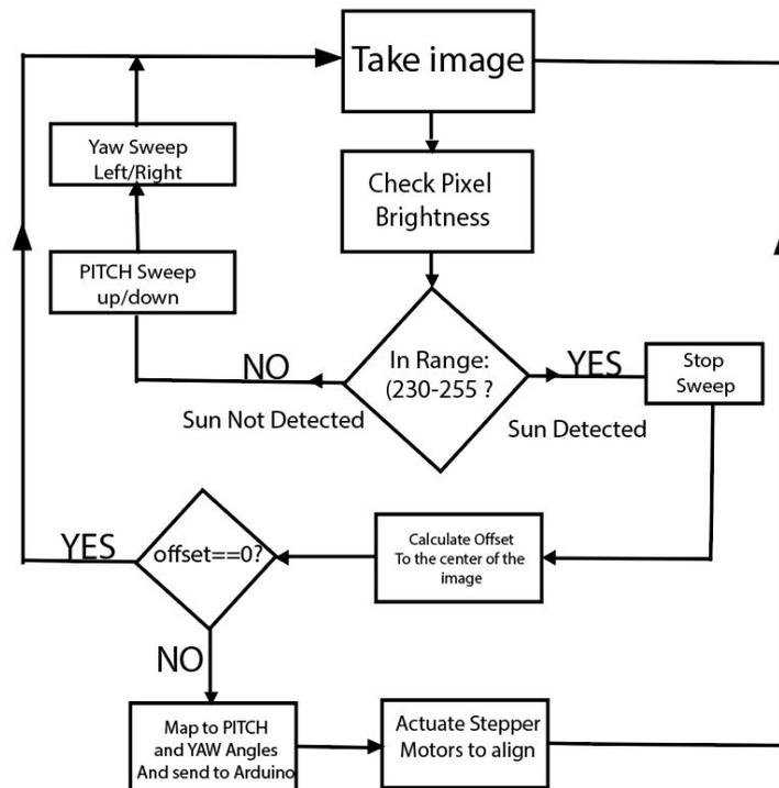
Figure 4.3.1.2.2 – Flowchart of the tracking algorithm
