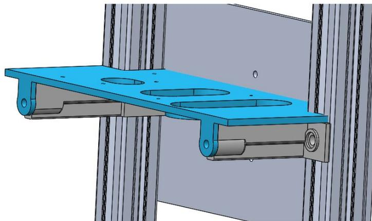
Figure 4.4.1.2 - SLM rails support acrylic trays to which electronics such as Arduinos were attached to directly via nylon standoff screws.
