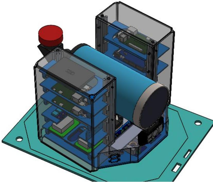
**Figure 9.4.1** - Component allocation inside the side E-boxes.
