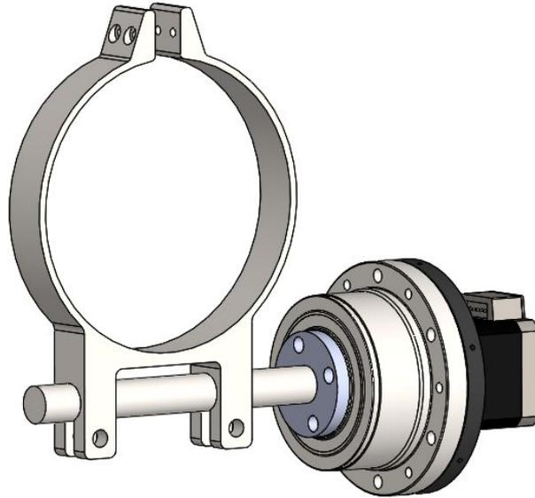
**Figure 4.3.6.2.2** - Motor, Bracket, Harmonic Drive, Shaft and Clamp Assembly.
