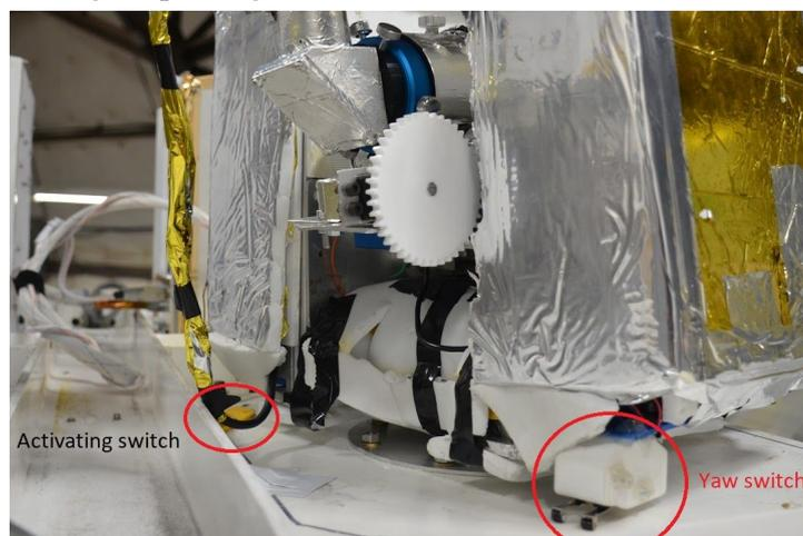
**Figure 4.3.6.2.5** - An activating switch was secured to the base plate, which activated the limiting switches when the gimbal rotates
