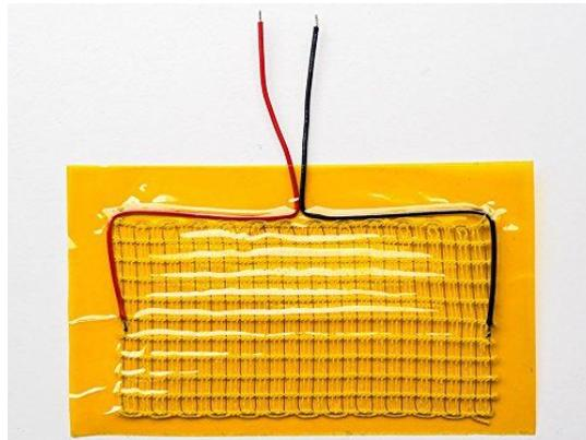
Figure 4.4.1 - Adafruit Electric Heating Pad
