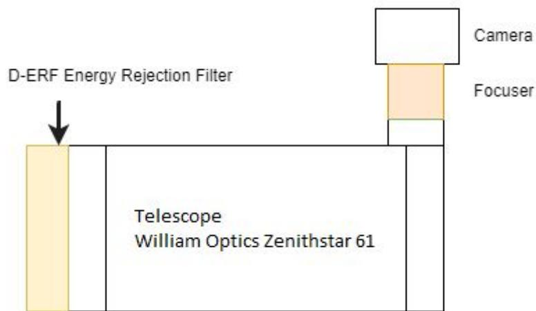
e 4.1.4.2 – Schematic of the final optical system
