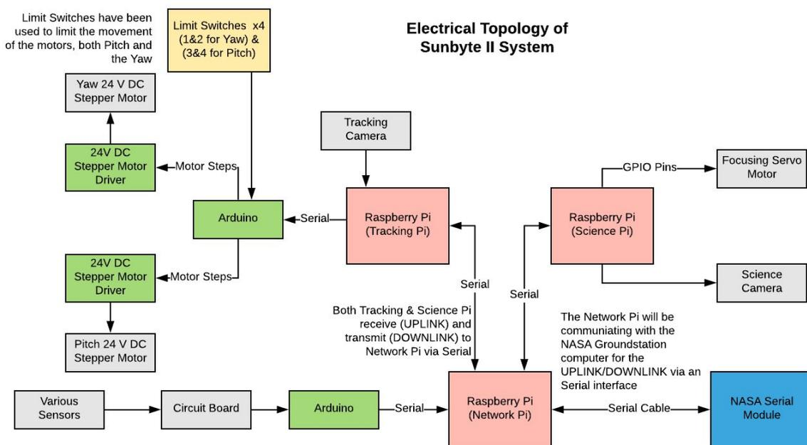
Figure 4.2.1.1 - Electrical Topology of the Sunbyte II system
