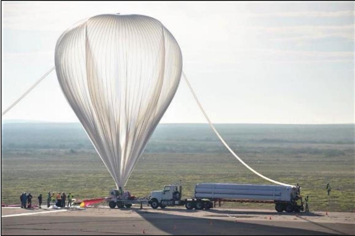
Fig.21(d) Inflating the balloon with helium gas.
