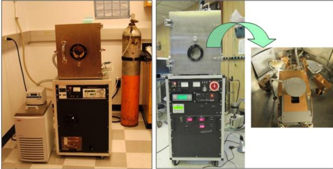
Fig. 3 (a) Thermal vacuum deposition system and (b) electron beam deposition system.
