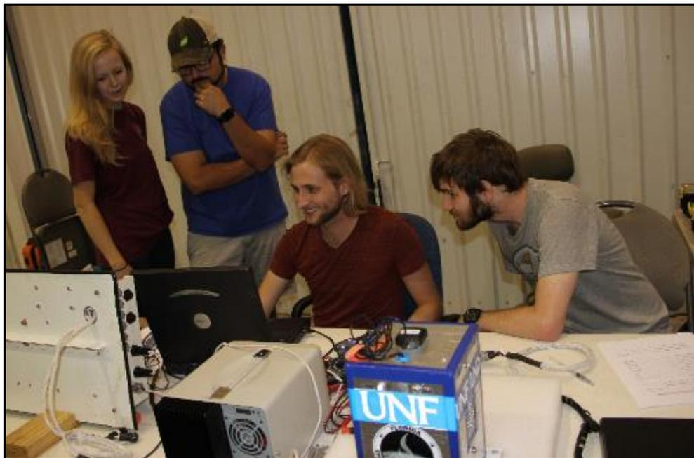
Fig.12 (a) Mr. Anthony Ficklin and Mr. Joshua Collins are testing of maximum current drawn by the UNF payload.
