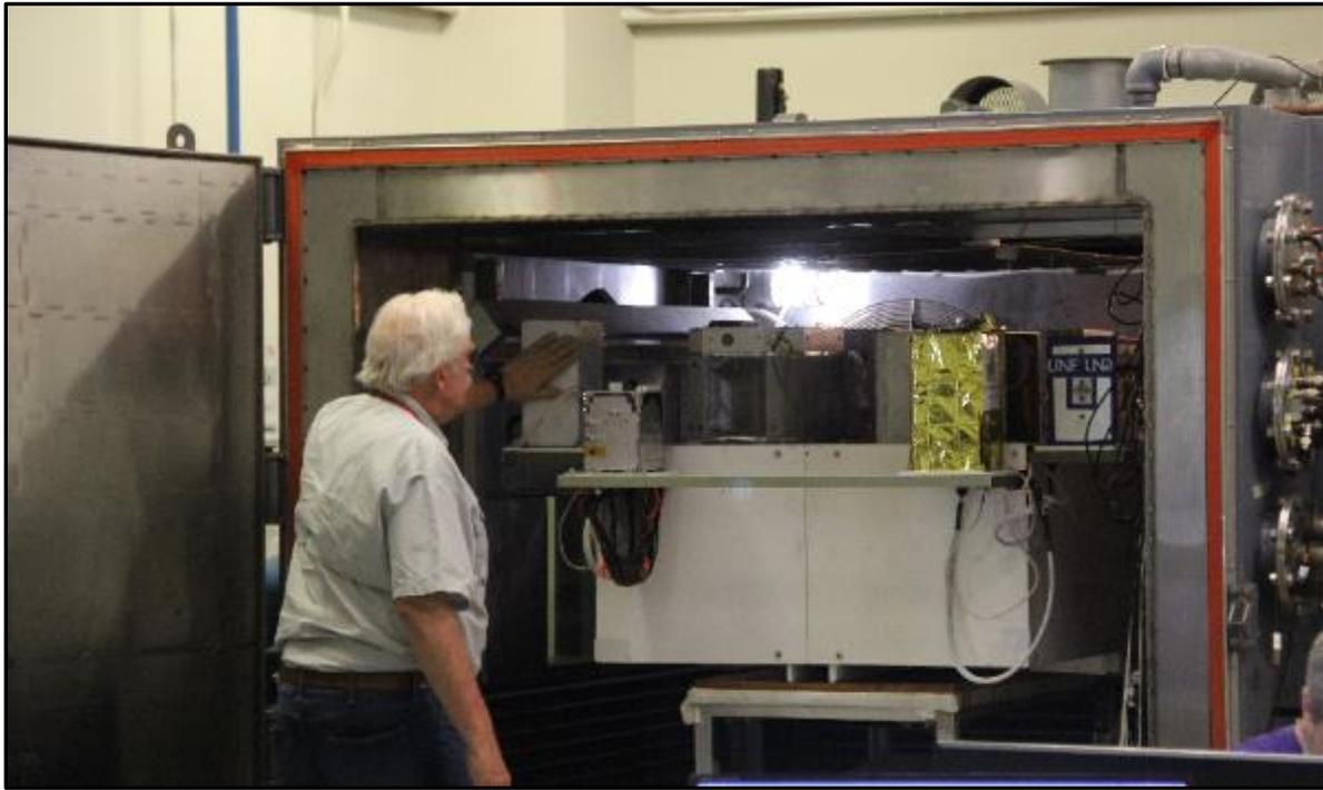
Fig. 19 (b) Inner view of a thermal vacuum test chamber shows stray light in the chamber and radiation heaters.
