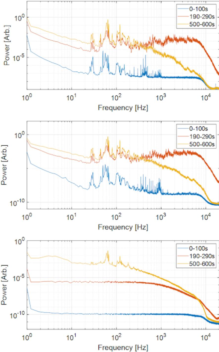
Figure 7: Power spectral densities for each identified time period for microphone 378A06 (top), 378B02 (middle) and 378A04 (bottom)
