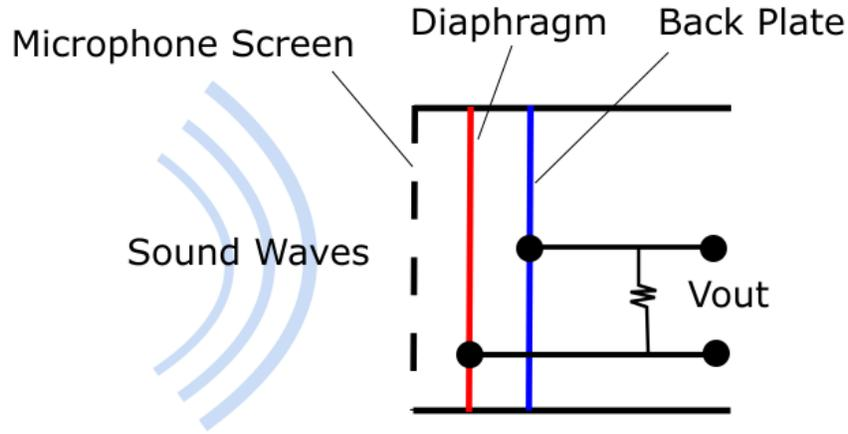
Figure 3: Microphone operating principle
