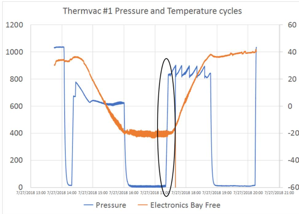
Figure 5: Pressure and temperature data from the first thermal vacuum test at CSBF with the region of interest circled
