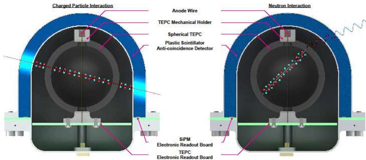
**Figure 1:** The CNP-TEPC instrument separates the dose from charged particles and neutrons by monitoring the signal from a hemispherical plastic scintillator Anti-Coincidence Detector (ACD), which surrounds a spherical TEPC detector. When charged particles interact with the instrument, shown on the left, they simultaneously deposit energy in the ACD and spherical TEPC. However, neutron interactions, shown on the right, deposit energy in one or the other but typically not both.
