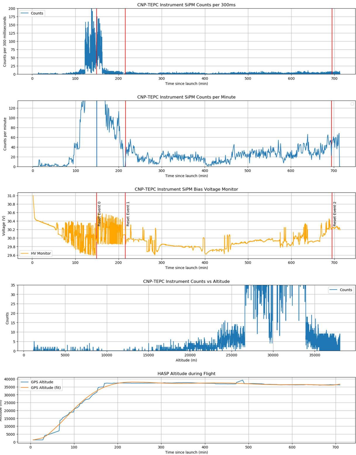
**Figure 16(A-E):** CNP-TEPC Instrument science data collected during the HASP 2018 balloon flight.
