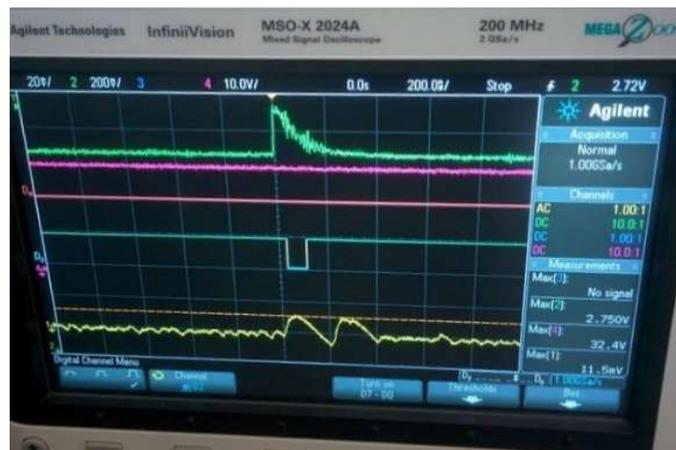
**Figure 2:** Lab Testing showing SiPM and CITIROC digital signals generated using Sr-90 + Y-90 source. Green signal is the raw SiPM Anode output, Blue signal is the CITIROC output trigger routed to the FPGA and Yellow is a CITIROC analog shaped output.
