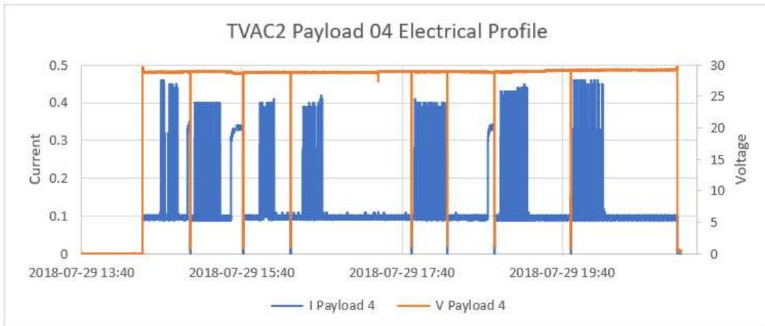
**Figure 9:** Payload voltage (orange) and current (blue) measurements during TVAC2. The spikes in current were due to the Communication Sub-System radio as the functionality of communications was being tested.
