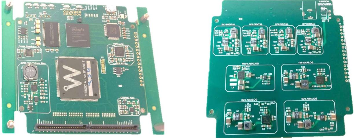
*Figures 3 & 4: Latest revisions of Data Acquisition and Power Distribution Boards respectively,*
