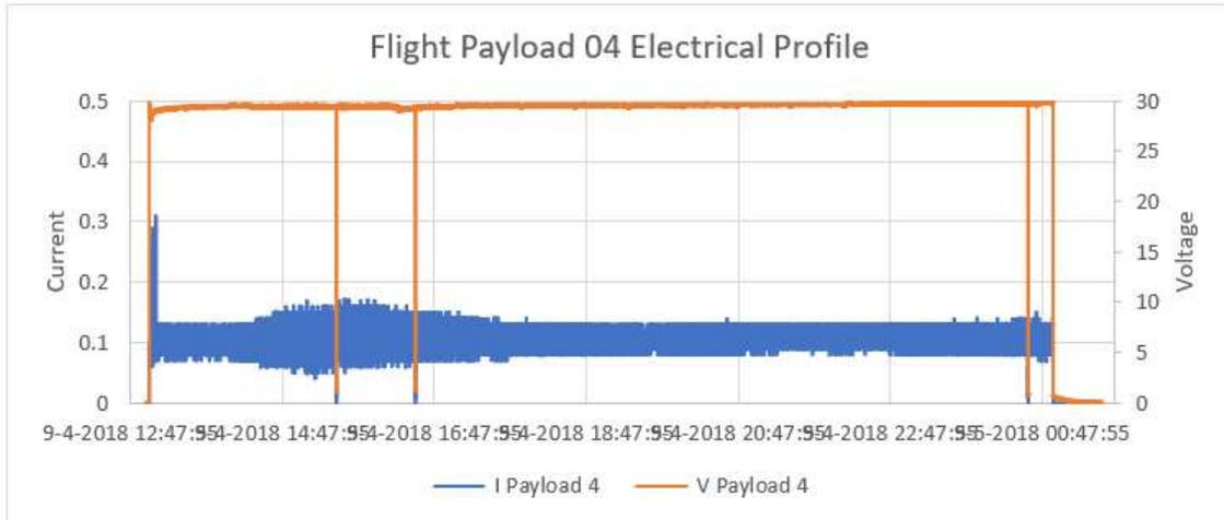
**Figure 10:** Payload voltage (orange) and current (blue) measurements during the HASP 2018 flight. The drops in voltage coincide to power cycles of the payload.
