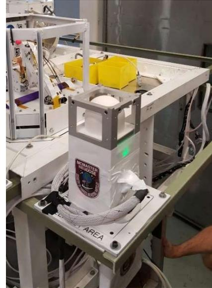
**Figure 8:** Payload successfully integrated onto HASP platform following a Thermal Vacuum Chamber Test.
