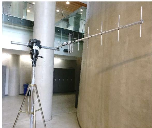
*Figure 5: Student designed and fabricated communications ground station*
