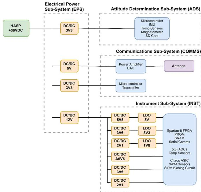
*Figure 6: Power Flow and System Block Diagram for the overall payload.*
