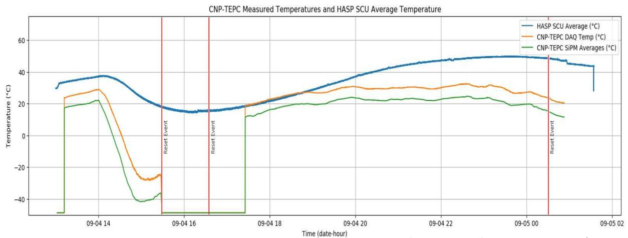
**Figure 11:** CNP-TEPC Instrument temperature measurements (orange and green lines) made during balloon flight. HASP’s SCU average temperature is also shown as the blue line.
