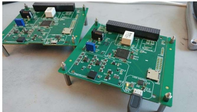
*Figure 7: Two ADS PCBs were assembled by the students, one for flight and one for validation.*
