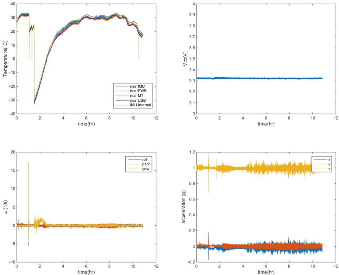
**Figures 12-15:** Data recorded on-board the Attitude and Determination Sub-System. Going clockwise starting from the top-left: Temperature Data, Supply Voltage Rail, Accelerometer Data, Gyroscope Data.
