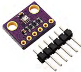
Fig. 21: For pressure and temperature, a single sensor is used: BMP280, flight proven on high altitude balloon missions throughout the world. https://www.makerfabs.com/index.php?route=product/product&product_id=295
