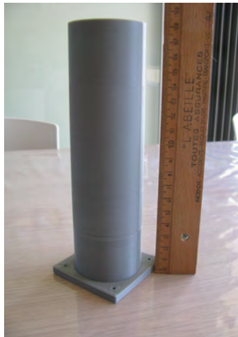
Fig. 19: The Gamma Spectrometer support structure, with base for securing it to the experiment structure. Standing 18,5cm tall, it houses the NaI crystal, the PMT and the \mu metal shielding. On top comes the HV supply and primary signal processing electronics [9].
