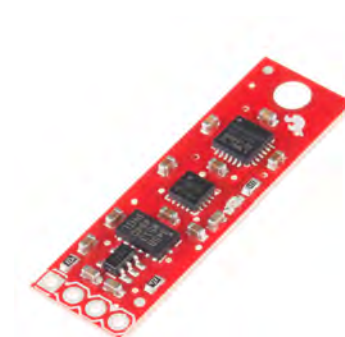
Fig. 22: The magnetometer is part of a 9 degrees-of-freedom inertial measurement unit: https://www.sparkfun.com/products/retired/10724 . It was flown successfully by our students on high altitude balloon missions from Brussels on several occasions
