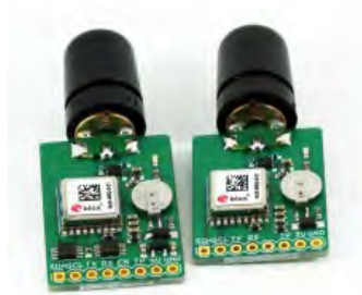
Fig. 20: The GPS module is Uputronics MAX M8 GPS module, flight proven on high altitude balloon missions in both the USA and the UK: https://store.uputronics.com/index.php?route=product/product&path=60_64&product_id=83
