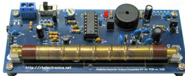
Fig. 3: The 3D Geiger counter is an assembly of 3 modules from RHElectronics: http://www.rhelectronics.net/store/radiation-detector-geiger-counter-diy-kit-second-edition.html
