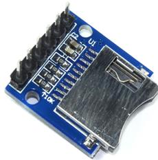
*Fig. 14 μSD card module for data storage. In use on our Arduino projects since 2015.*
