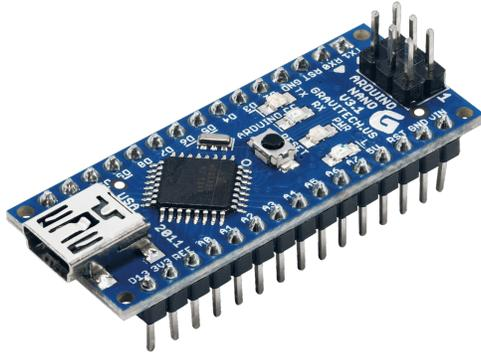
*Fig. 13 Arduino Nano microcontrollers are used on all experiments except the gamma spectrometer, where the data rate and data processing complexity require the Raspberry Pi 3's (or Raspberry Pi Zero's) vastly greater capabilities.*
