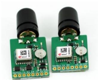
*Fig. 10 The GPS module is Uputronics MAX M8 GPS module, flightproven on high altitude balloon missions in both the USA and the UK: [https://store.uputronics.com/index.php?route=product/product&path=60\\_64&product\\_id=83](https://store.uputronics.com/index.php?route=product/product&path=60_64&product_id=83)*
