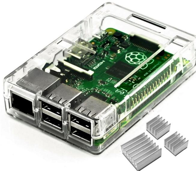
*Fig. 8 The Raspberry Pi3 controller will run a Linux kernel, WINE and PRA as dedicated gamma spectroscopy software, and homebrew software for data storage.*
