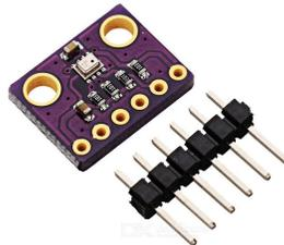
*Fig. 11 For pressure and temperature, a single sensor is used: BMP280, flight proven on high altitude balloon missions throughout the world.
