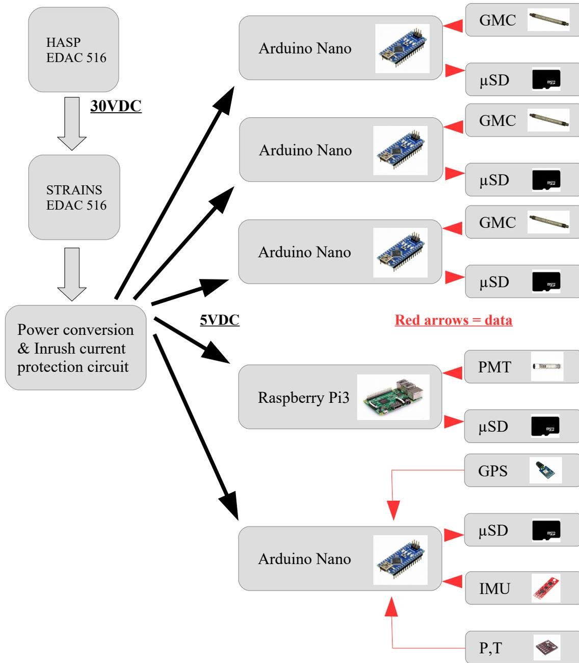
Fig. 4 Payload System Diagram
