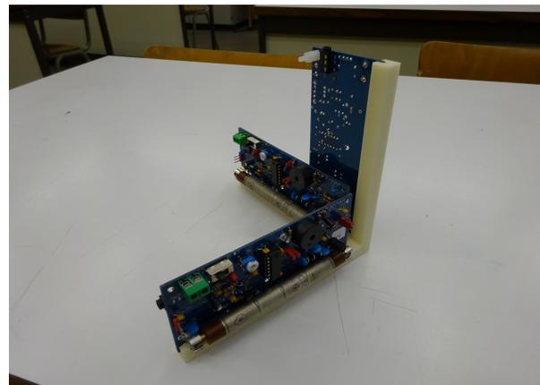
*Fig. 17&18 A 12x12x12 cm 3D printed ABS frame holds the Geiger counter modules in place, their tubes neatly perpendicular to one another. Each Geiger counter is connected to an Arduino Nano that carries a  $\mu$ SD card module for data storage. This arrangement will have to be modified to ensure a nice fit within the aluminum structure, and to optimize the use of available space.*
