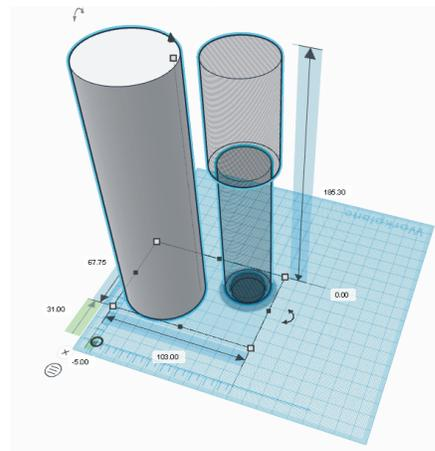
*Fig. 15&16 The hollow casing aligning the photomultiplier tube (and its mu-metal shielding) and the NaI scintillation crystal under development. A suitable base will need to be added to allow the setup to be properly secured to the experiment's base plate.*
