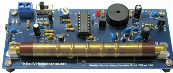
*Fig. 9 The 3D Geiger counter is an assembly of 3 modules from RHElectronics:
