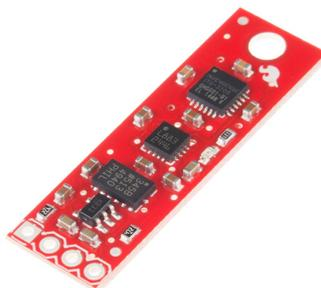
*Fig. 12 The magnetometer is part of a 9 degrees-of-freedom inertial measurement unit:
