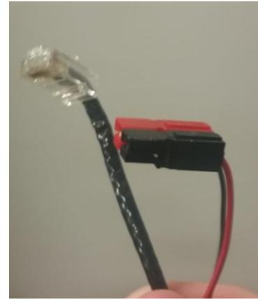
Figure 4: Cable terminations used for supplying power the M5 (left) and the Micro-Trak (right).
