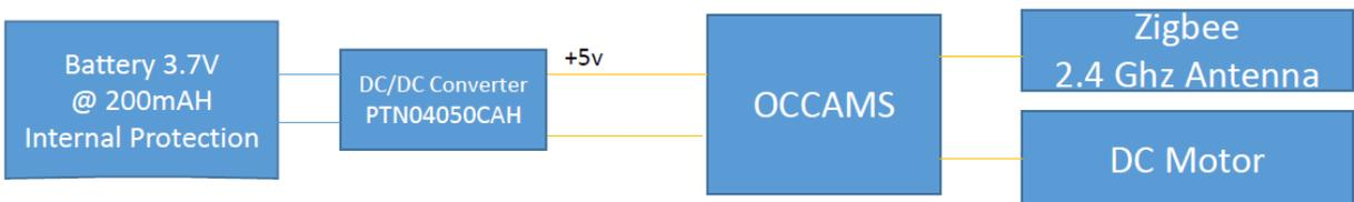
Figure A5: Termination System Block Diagram
