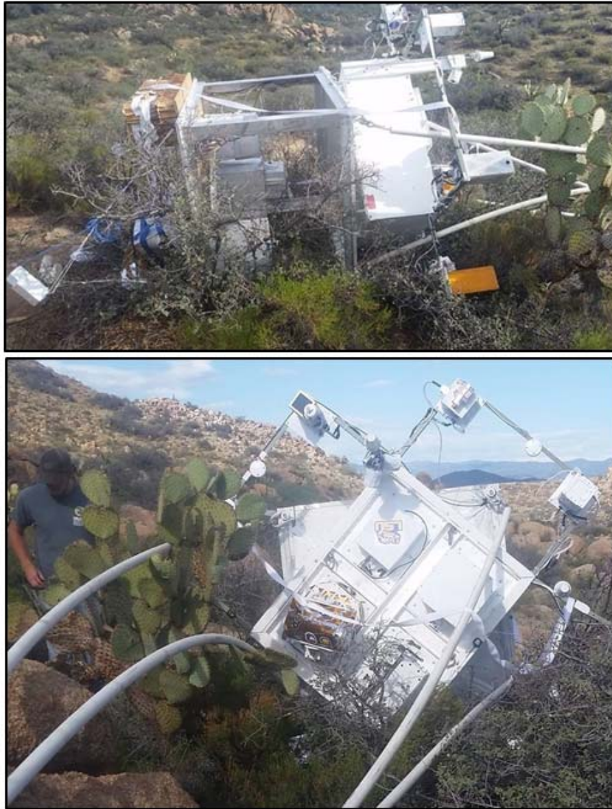
Fig. 23 (a) Impact of HASP on the ground.
