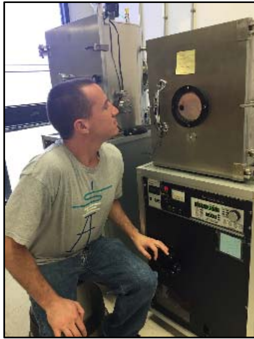
Fig.8 (n) Chris operated the high vacuum systems for the fabrication of thin film gas sensors.
