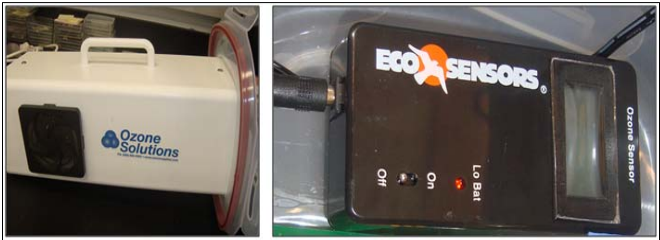
Fig.6(a) Ozone generator and (b) digital ozone detector.
