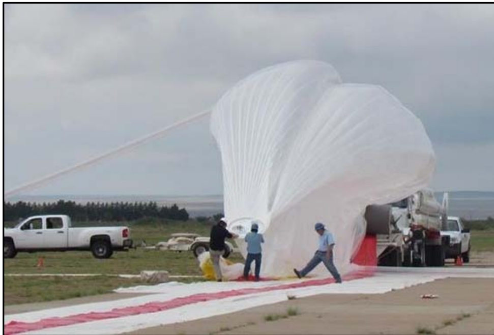
Fig.21(d) Inflating the balloon with helium gas.
