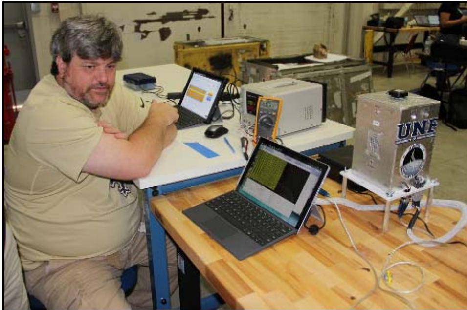
Fig.12 (a) shows Dough is testing of maximum current drawn by the payload.
