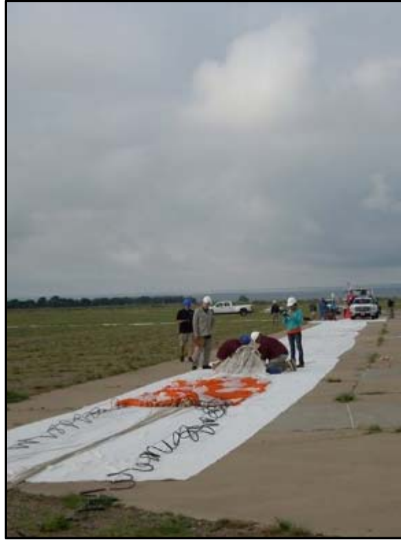
Fig. 21(c) Launch preparation and attaching the parachute with the HASP.
