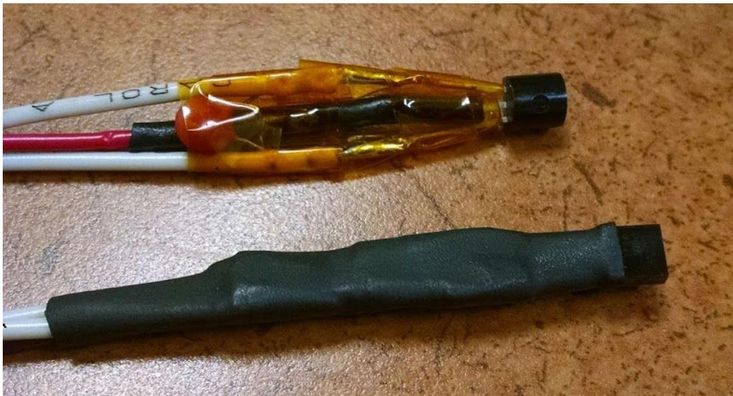
**Figure10.** TMP36 temperature sensor internals
