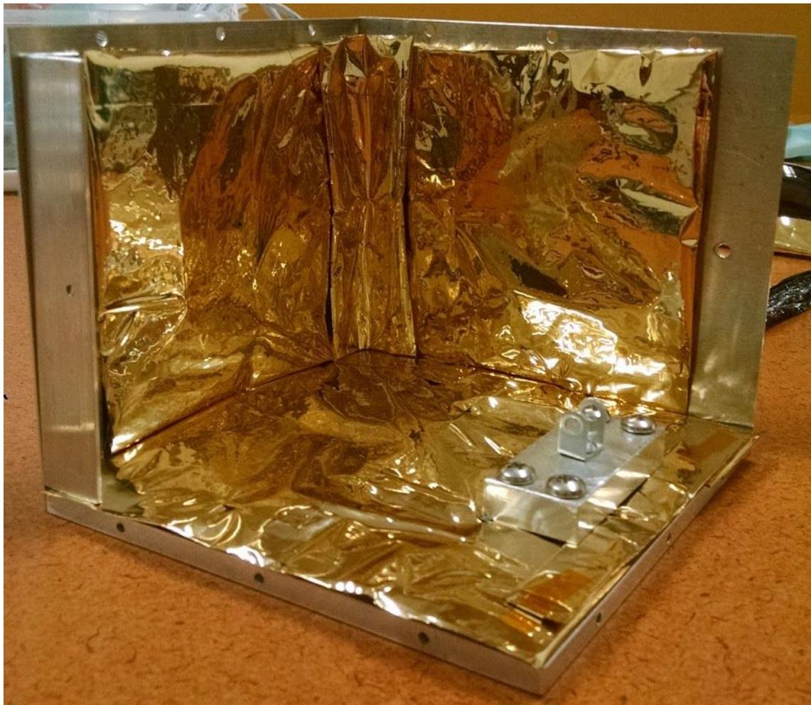
**Figure8.** Reflective mylar and aerogel blanket insulation used in the PTC system
