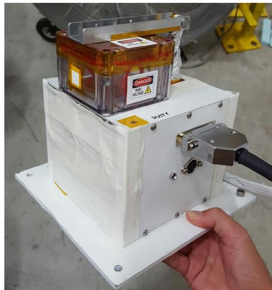
**Figure2.** Flight-ready ECDC Payload (Aug. 2016)
