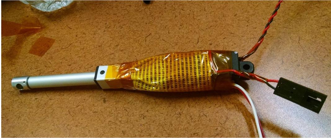
**Figure9.** Actuator with heating pad and temperature sensors installed
