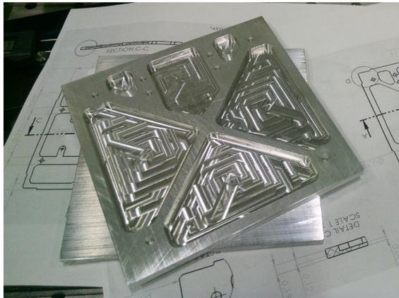
**Figure4.** CNC-milled bottom support plate
