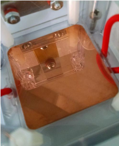
**Figure 23a.** Flown copper plate collector during analysis
