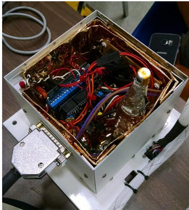
**Figure6d.** Assembled flight payload with flight components and insulation
