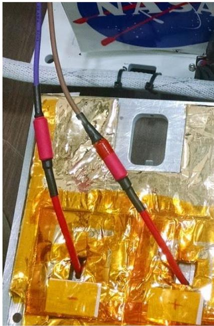
**Figure7a.** High voltage splice insulation
