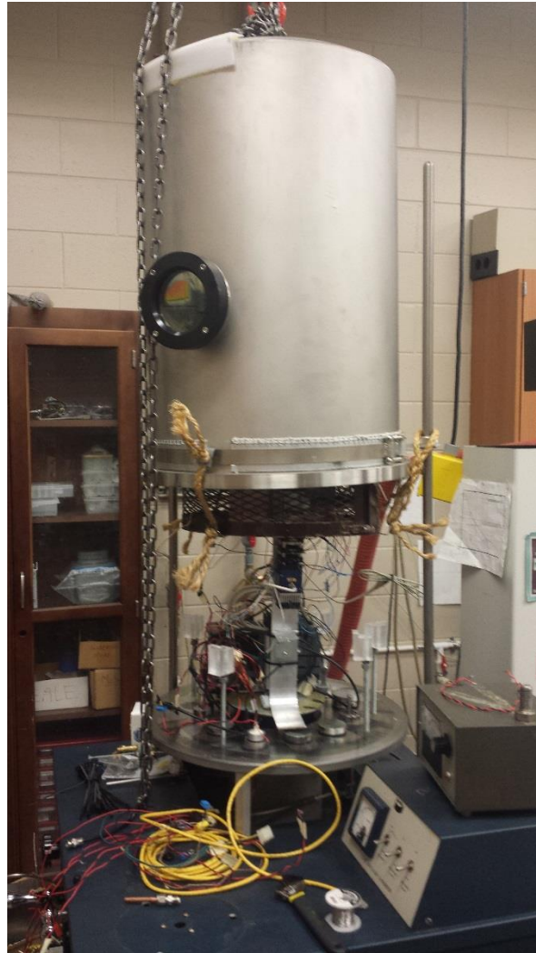
Figure 3: Temporary minimal chassis for ease of system electronics modification inside of opened Environmental Chamber
