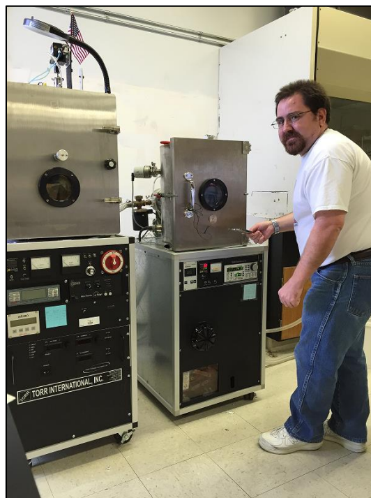
Fig.4 Joe is operating the high vacuum systems for the fabrication of thin film gas sensors.
