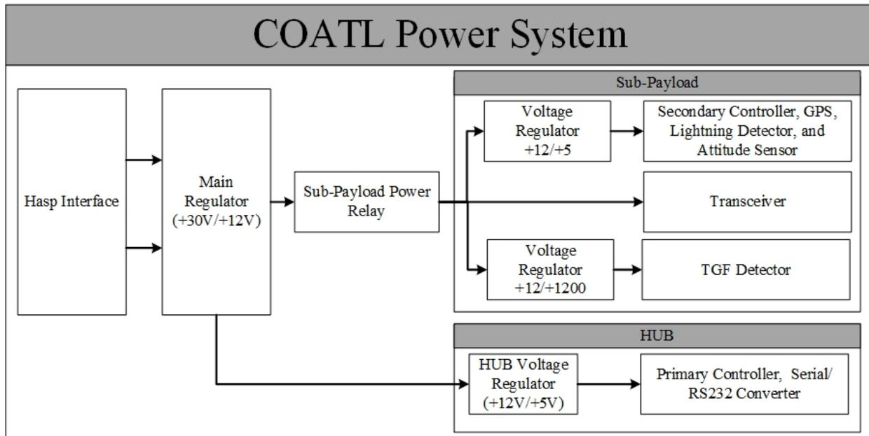
Figure 7: Power System Diagram
