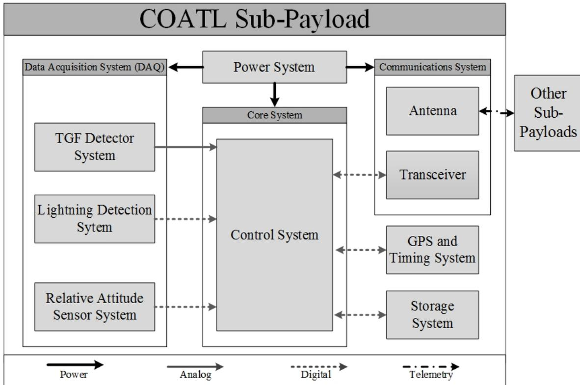
Figure 5: High Level System Design for each Sub-Payload
