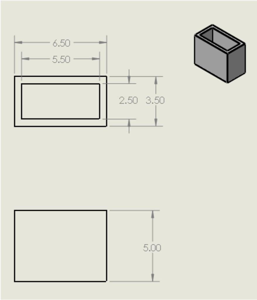
Figure 19: Central HUB detail with dimensions in inches. The Central HUB is primarily composed of 0.5'' thick Polystyrene foam.
