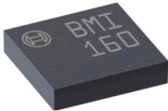
*Figure 11: BMI160 IMU Chip*
