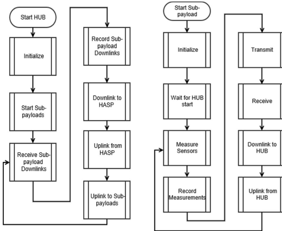
Figure 13: High Level Flight Software Flowchart for HUB and Sub-Payload
