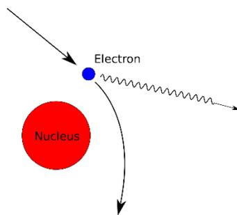
Figure 2: Diagram of gamma-ray emission from Bremsstrahlung.
