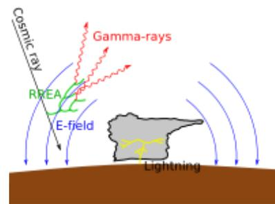
Figure 1: Diagram of a TGF production mechanism.
