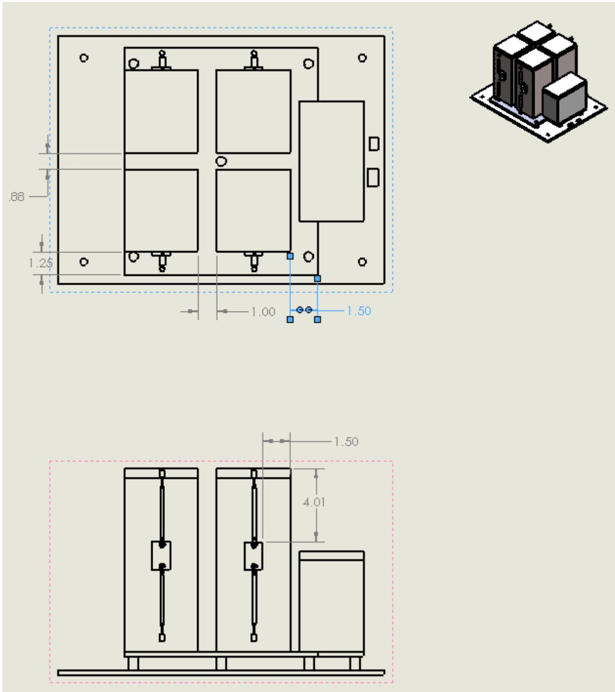
Figure 20: Full Payload Assembly drawing detailing antenna and payload box placement and the payload footprint on the HASP plate. Dimensions in inches.
