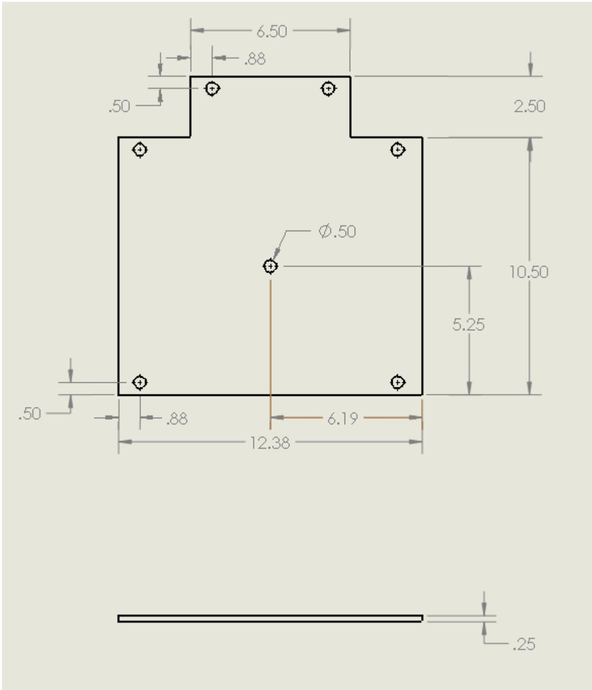
Figure 21: Mounting Plate detail with dimensions in inches. The mounting plate is composed of PVC.
