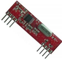
*Figure 10: RF Solutions QAM-RX5-433-ND AM Modulator*
