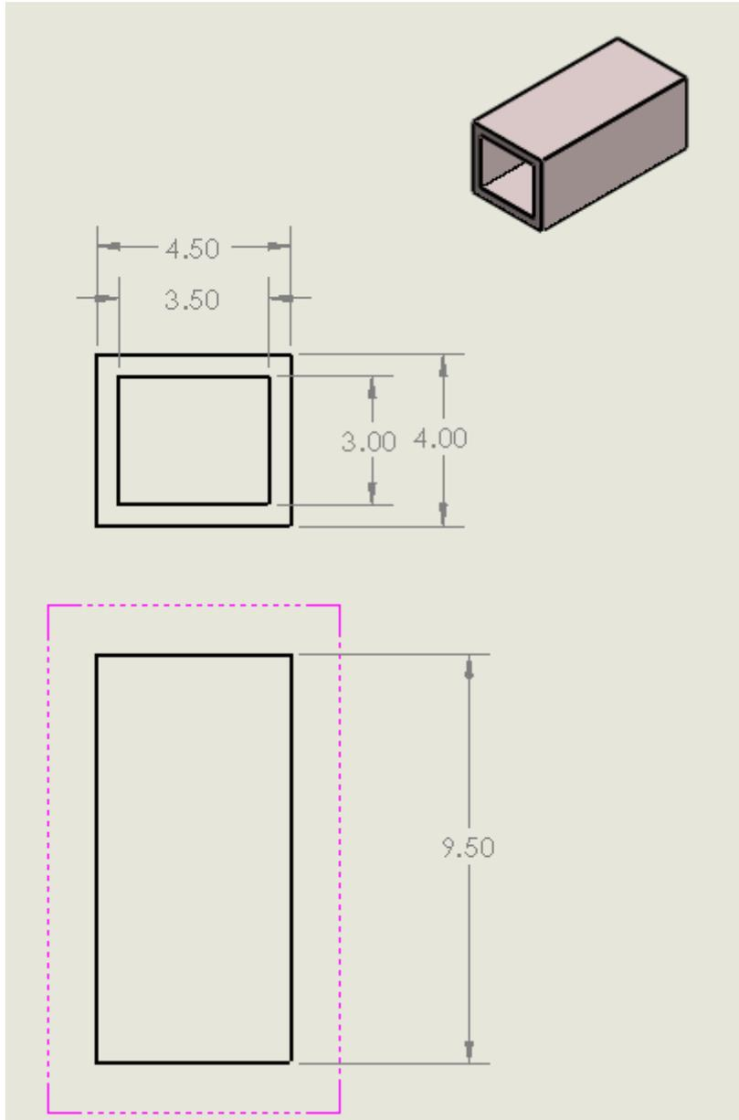
Figure 18: Payload Box detail with dimensions in inches. The Payload Boxes are primarily composed of 0.5'' thick Polystyrene foam.
