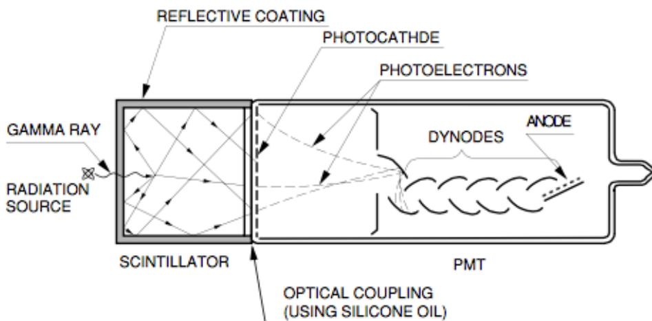
Figure 8: Scintillator and PMT coupling
