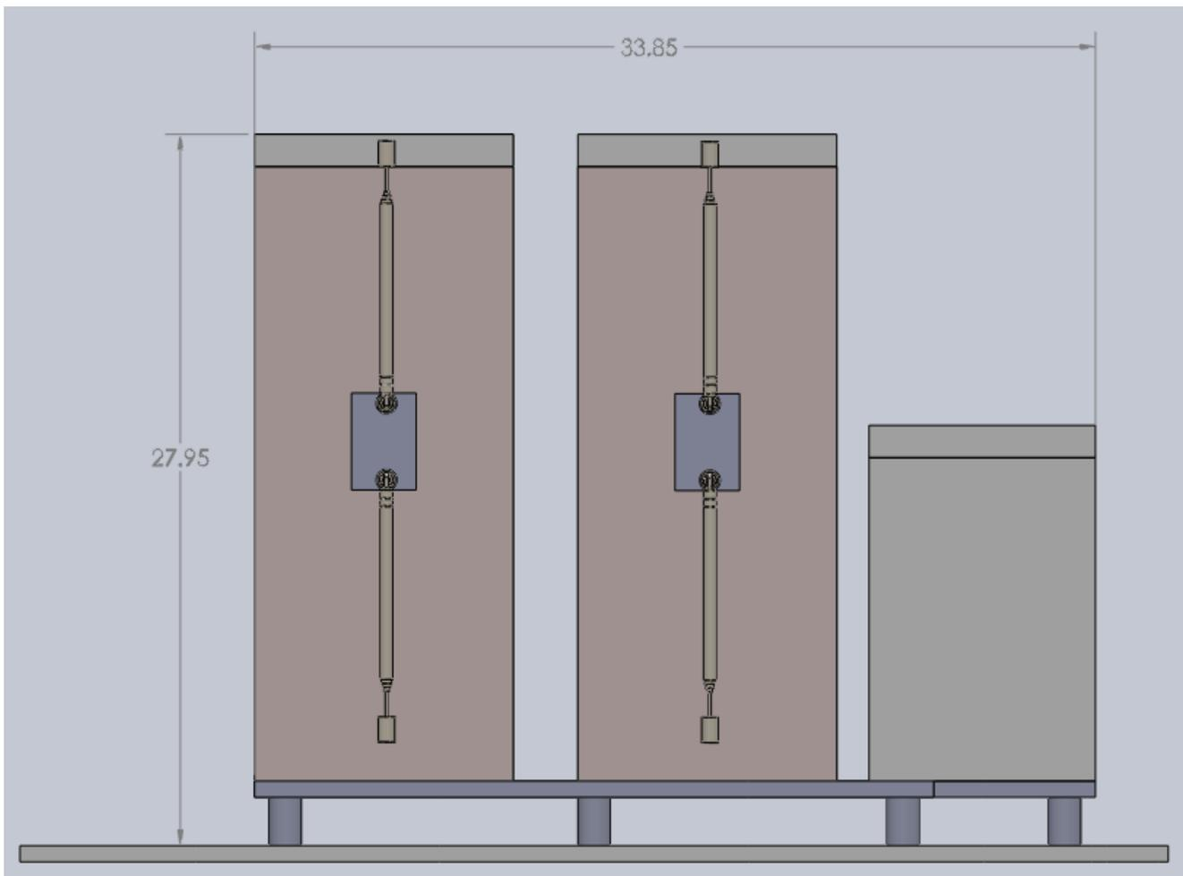
Figure 16: 3D rendering of the side view of COATL. COATL is 27.95 cm (11 in) tall, which fits within the maximum allowed height of 30 cm. COATL is 33.85 cm (13.33 in) long, which fits within the maximum allowed length of 40.32 cm (15.875 in).
