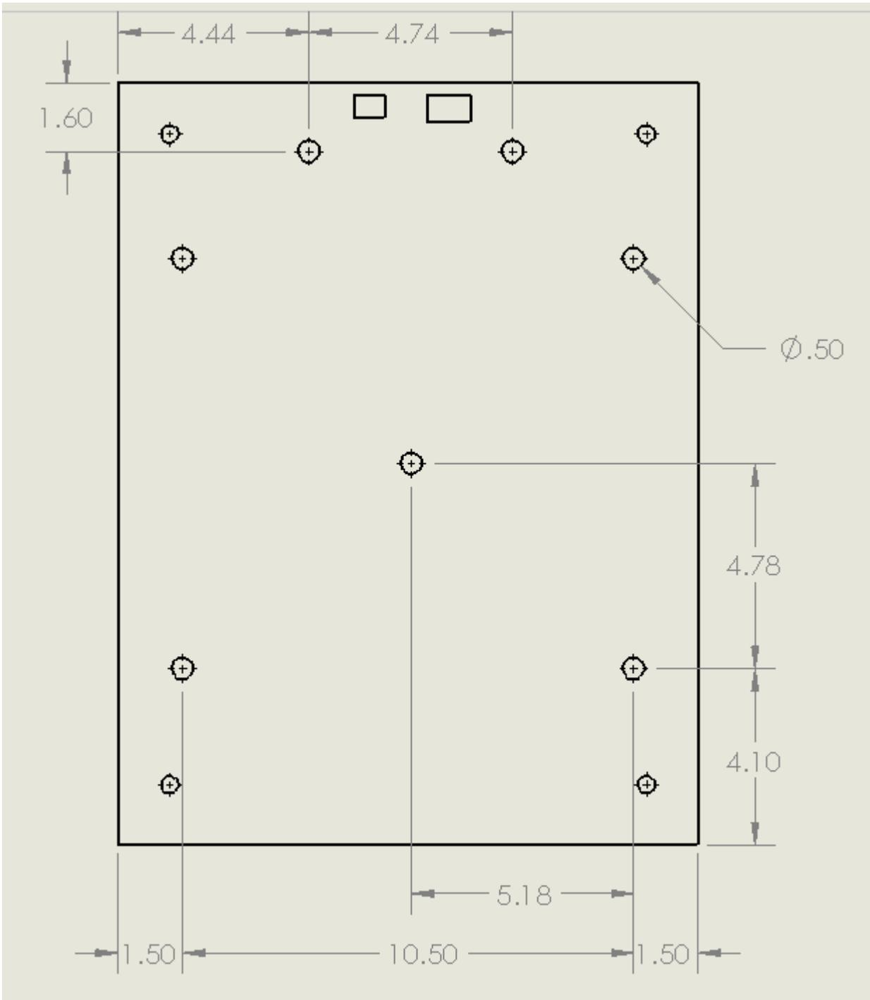
Figure 17: Anticipated HASP mounting plate modifications. Seven holes will be drilled in order to mount the payload. All of the drilled holes will be 0.5 inches in diameter. (units in inches)
