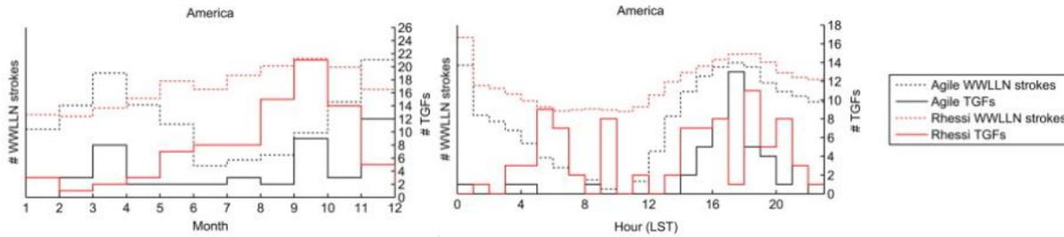
Figure 3: TGF Production Cycles shows the recorded TGFs and lightning strikes measured over the American tropics by AGILE and RHESSI for March 2009 – July 2012 distributed by month and diurnal time (Fabr3, Ferran).
