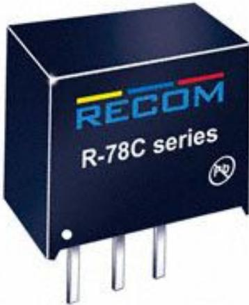
The 5V converter to be used is the Recom Power R-78C5.0-1.0 . This converter takes an input voltage of +8-42Vdc and converts it to +5Vdc at 93% efficiency. It outputs a maximum current of 1A and a maximum power output of 5W. The converter is temperature rated between -40°C and 85°C.
