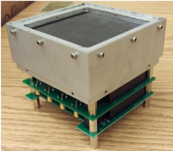
**Figure 4.** Gamma Ray Incidence Detector (GRID).
