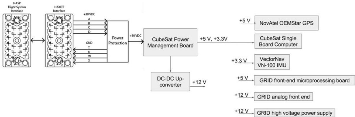
**Figure 6.** Shown is a high-level block diagram of the payload power distribution system. The power management board features two regulated power buses: 3.3V@5A and 5V@4A. Additionally, a +12V rail will be derived via a DC-DC converter.
