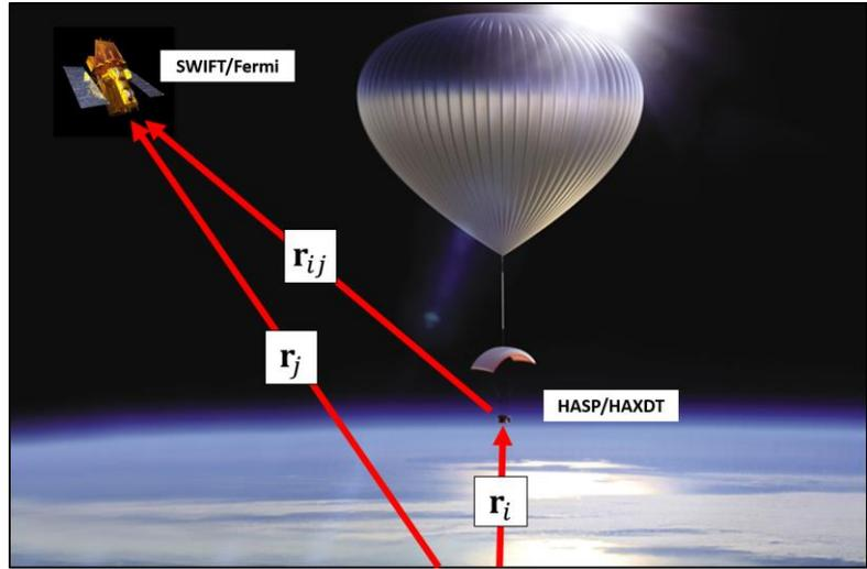
**Figure 1.** Concept of operation for testing the ranging and timing functions of GRID if a Gamma Ray Burst (GRB) even it observed during float.
