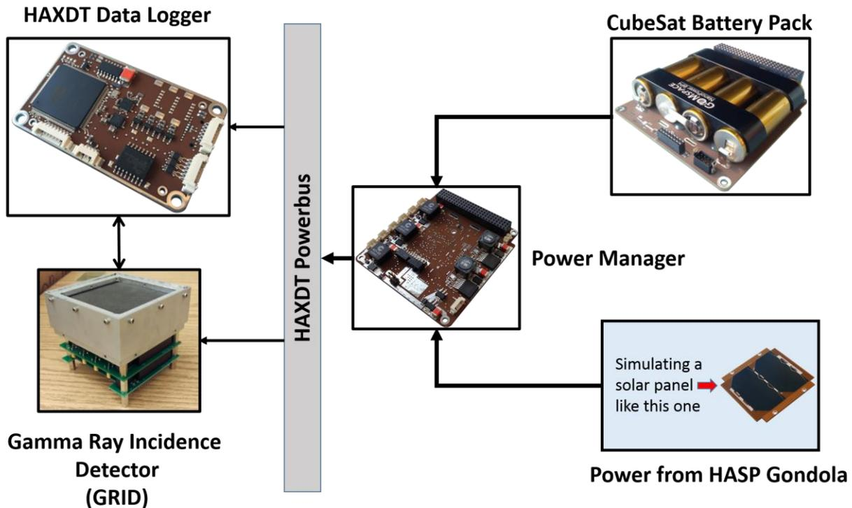
**Figure 2.** Schematic of hardware system that will be tested on HAXDT during the 2016 HASP flight.
