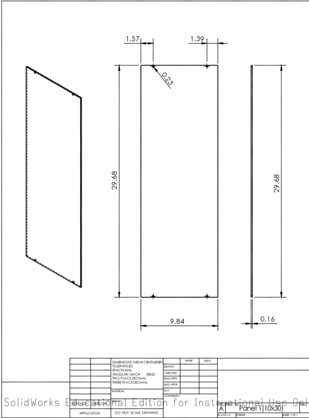
**Figure 8.** A mechanical drawing of the aluminum side panels of the 3U CubeSat structure, with dimensions in centimeters.
