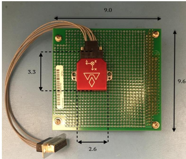
**Figure A11.** VectorNav VN-100U, shown sitting on top of a PC/104 prototype board for scale
