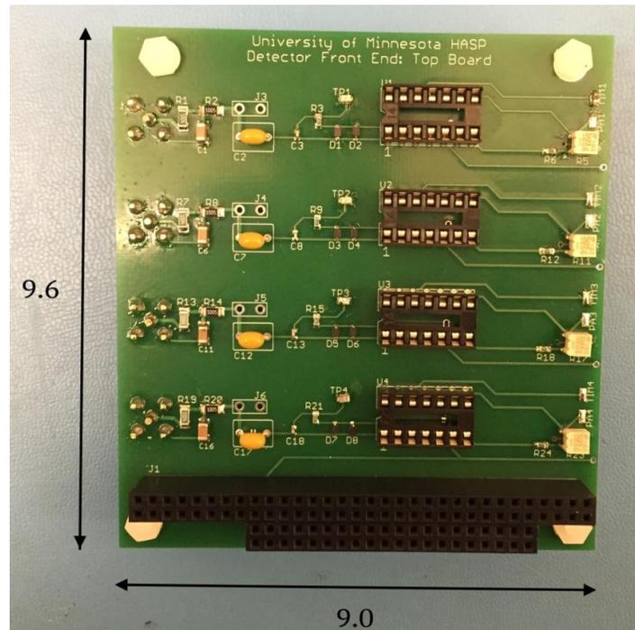
**Figure A9.** Custom-designed four-channel detector front end board, with dimensions in centimeters. This board will house the Amptek A225 charge-sensitive preamplifier chips (not populated here). A second front end board, not yet completed, will house both the Amptek A206 amplifier/discriminator chips and the peak detector circuits for photon energy measurement.
