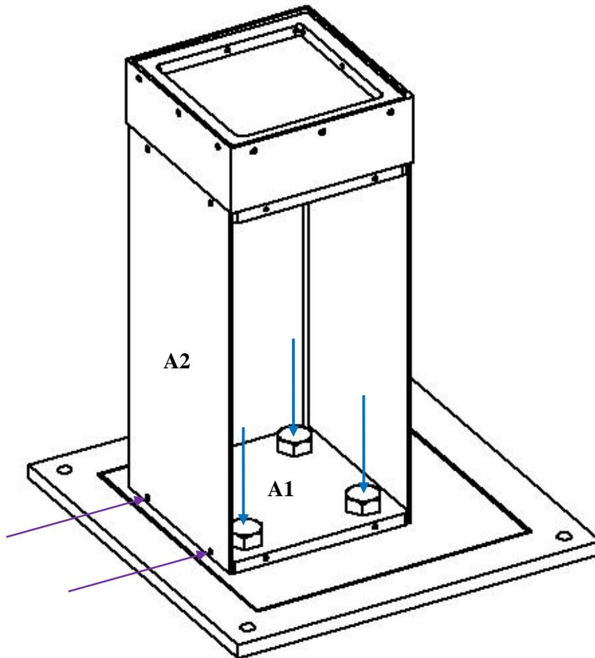
**Figure A7.** Mechanical drawing of the U-shaped panel (A2) attached to the bottom plate (A1) via screws located at the purple arrows going horizontal to the HASP mounting plate. There will be 2 of these screws on each side of A2 as well as on the access panel (A3, not shown). A1 is attached to the HASP mounting plate by 4  $\frac{1}{4}$ " diameter bolts shown by the blue arrows going perpendicular.
