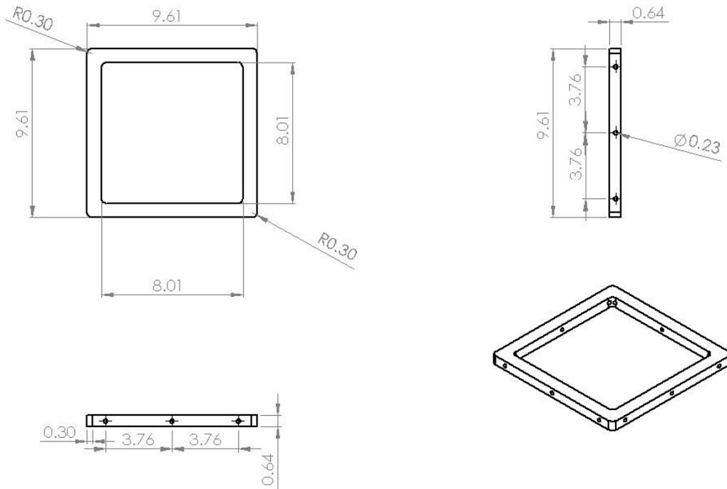
**Figure A6.** Mechanical drawing of detector window clamp given in centimeters. This part will sit inside the detector housing, above the detector window, and will hold the window in place without the need for rigid attachment of the carbon fiber. It will also serve to press the window into the detectors, holding them firmly in place in their foam-lined enclosures in the detector housing.
