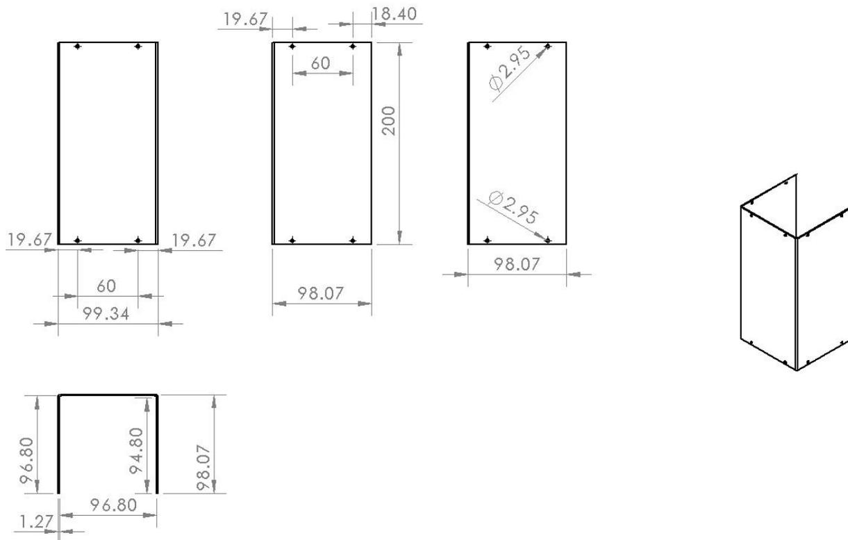
**Figure A2.** Mechanical drawing of the U-shaped load bearing structural wall with dimensions in millimeters. This wall is bent from a single sheet of 5052-H32 aluminum. The HASP power and downlink signals will also be routed through a connector in this wall, which is not shown here. The walls will have an outer cross section of 10x10 cm in order to simulate CubeSat constraints.
