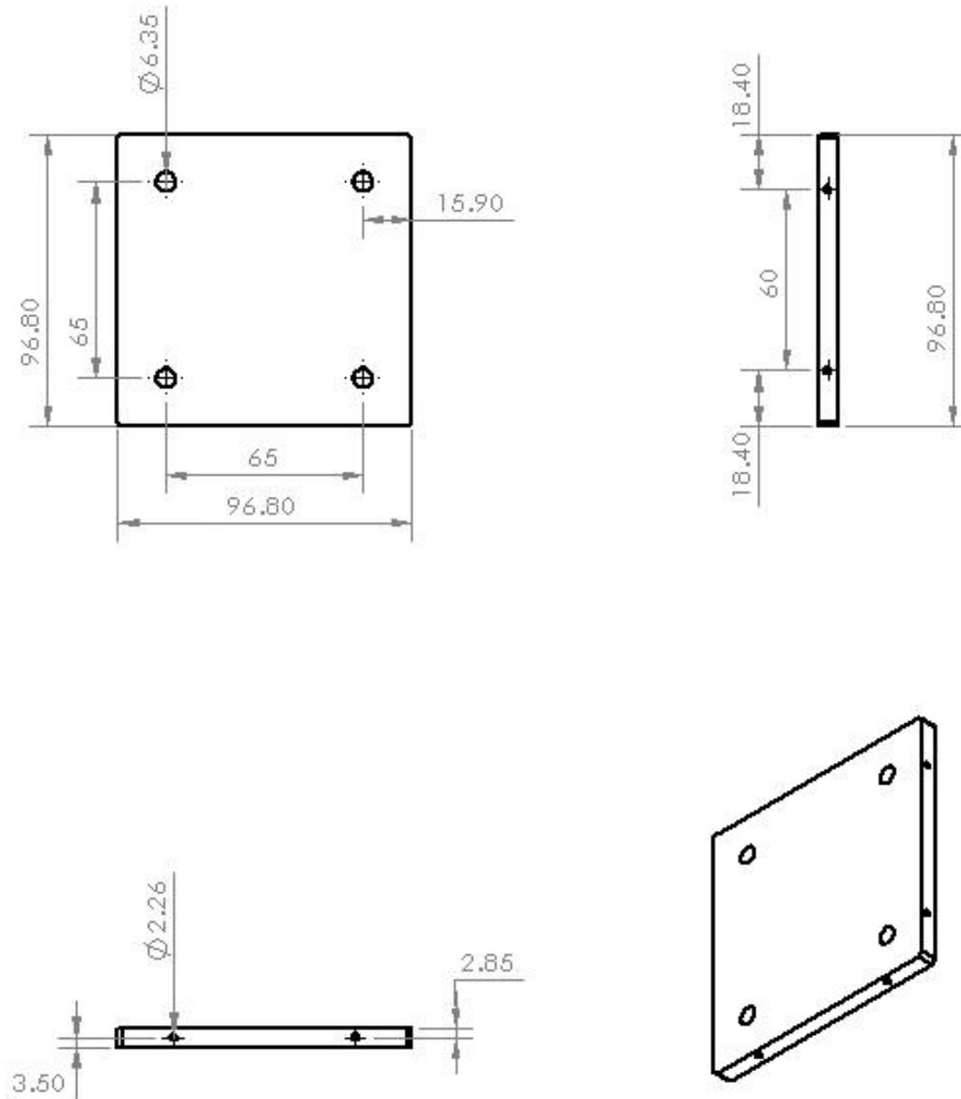
**Figure A1.** Mechanical drawing of the bottom plate of the structure with dimensions in millimeters. This plate attaches to the HASP mounting plate using  $\frac{1}{4}$ -inch diameter bolts and serves as the anchor for the U-shaped wall and access panel (see Figure A2, A3 respectively).
