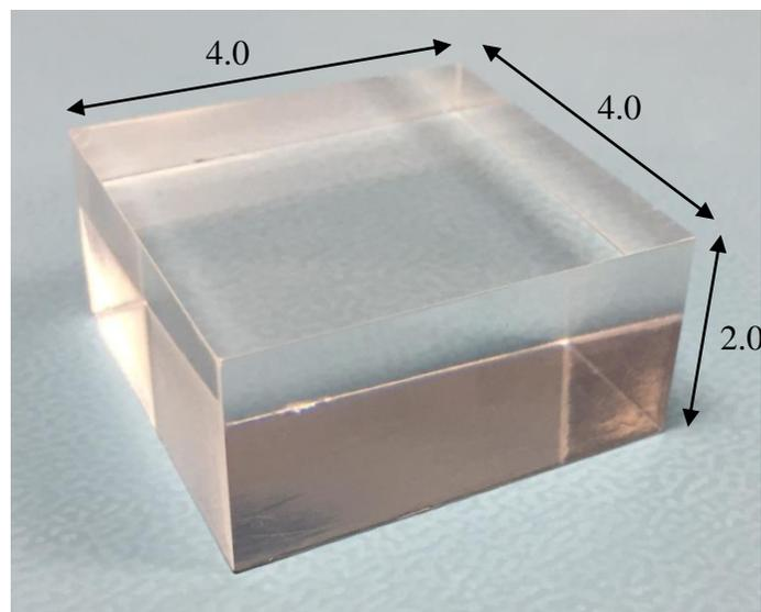
**Figure A10.** Thallium-doped cesium iodide scintillation crystal with dimensions in centimeters. One of these crystals will be used in each of the four detectors.
