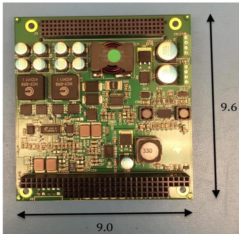
**Figure A15.** WinSystems PPM-DC-ATX-P power supply board with dimensions in centimeters.
