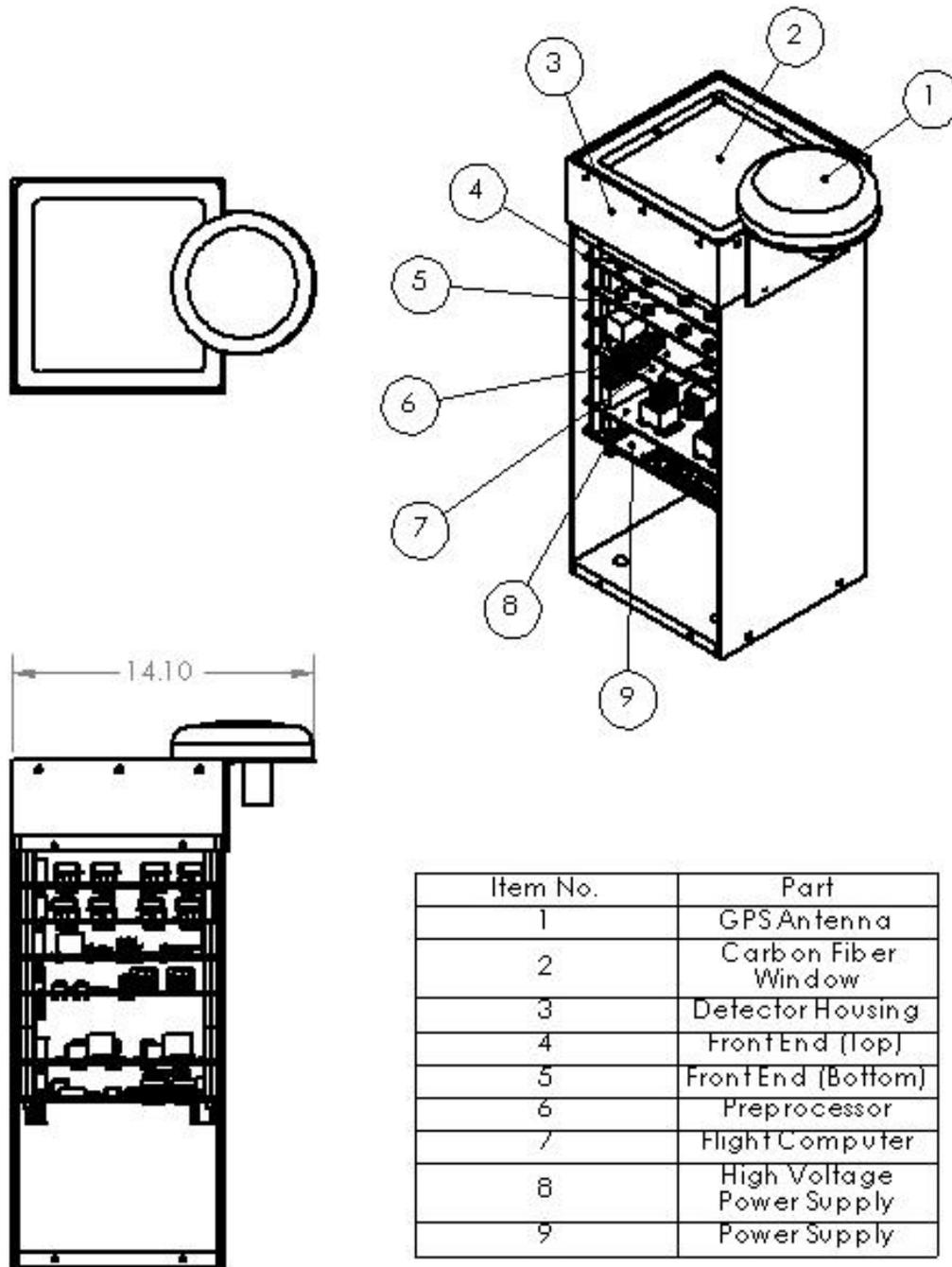
**Figure A8.** Mechanical drawing of the full payload assembly given in centimeters. The access panel is hidden in this viewing, showing the full stack of electrical components suspended from the detector housing. Parts are numerically annotated in relation to the table provided:
