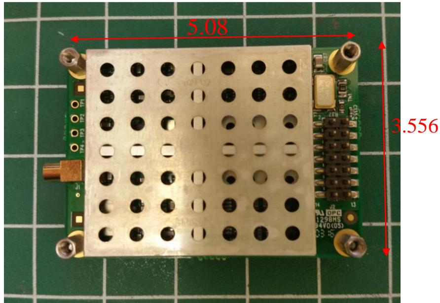
**Figure A14.** Picture of the FreeWave MM2-T radio transceivers with measurements given in centimeters. The dimensions are 5.08 L x 3.556 W x 0.95 H (cm).
