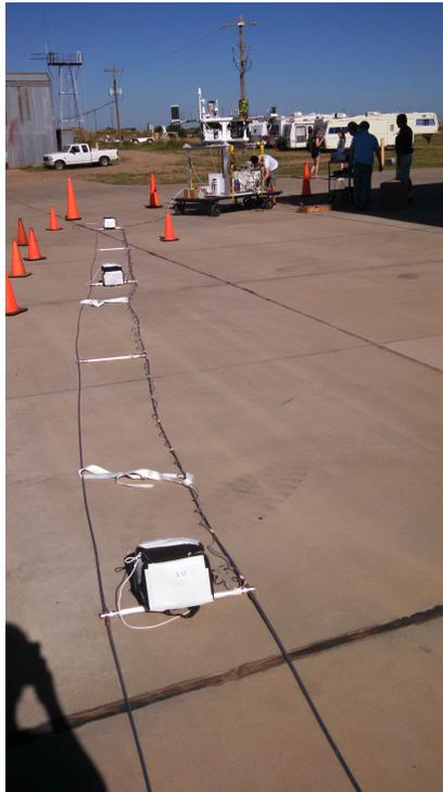
Figure 2: Microphones enclosed in lunch coolers and attached to the flight ladder. This ladder runs between the gondola and the parachute during flight.
