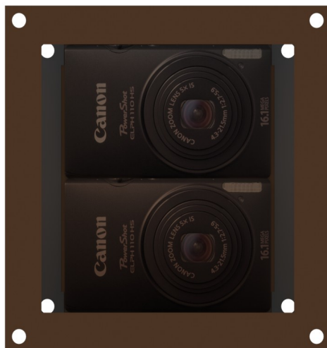
Figure 6. Bottom view, cameras recessed - this is the side of the instrument that will be bolted to the HASP plate and viewing holes will need to be cut out of the HASP plate.
