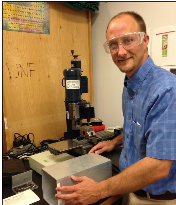
Fig.1 Ken Emanuel (UNF) is working over the fabrication of payload using the Desktop CNC Machining System, Model: Micromill 2000, http://www.microproto.com/micromill2000.htm
