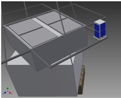
The picture below allows to get a better view of how the payload is connected to HASP with the use of nuts and bolts:
