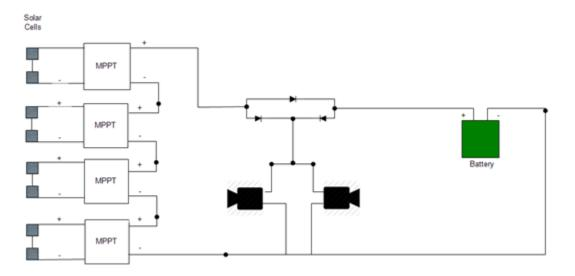
The three-diode system acts as a controller among the three parts: it provides power to the battery to charge when its level is low, avoids current to feed back to the solar cells and let current flow to the cameras.
