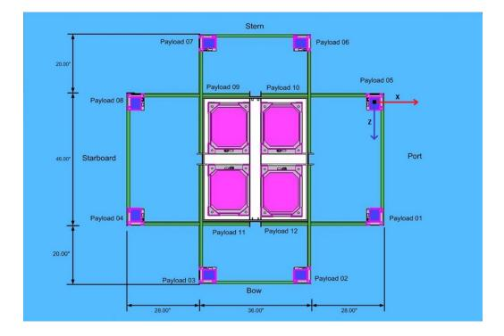
Looking at Payload 05 in the drawing above, it can be seen that the side of the payload with the side-facing camera will be pointed along the x-axis to obtain an unobstructed view of the surroundings. The side of the payload with connectors will be facing HASP directly (opposite direction of the x-axis).
