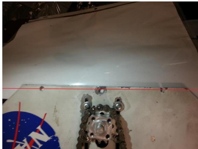
**Figure 6.5.0 Misaligned Screw Holes.** *The top plate holes to connect to the side panels were made incorrectly*
