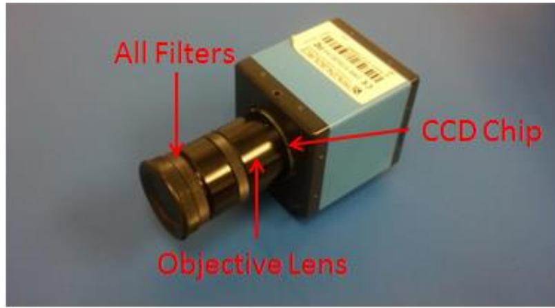
Figure 4.1.2 ADCS Camera
