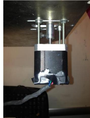
**Figure 4.3.6 X axis motor. 68 oz. stepper motor. Motor was attached under the HELIOS II top plate**
