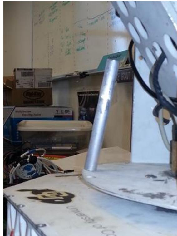
**Figure 5.5.1 Bent circular plate.** *The circular plate underneath the camera housing was bent during the HASP landing.*
