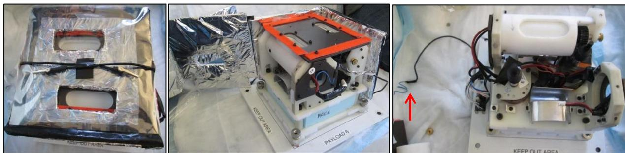
**Figure 4) Left to Right: 1.** Canisters closed upon landing; **2.** Payload without thermal insulation; **3.** Payload without canister 2. The red arrow indicates the loose ground wire from Canister 1
