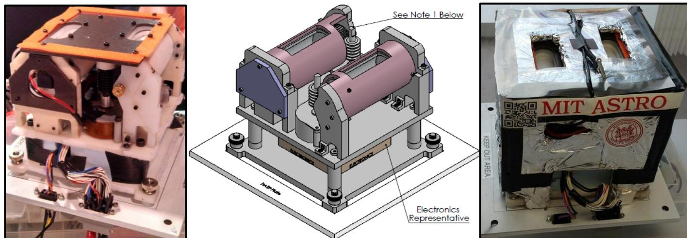
**Fig 1) From left to right** – 1) Assembled payload without thermal insulation ; 2) SolidWorks rendering of system ; 3) Completed payload with mylar & foam thermal insulation and static dissipative film
