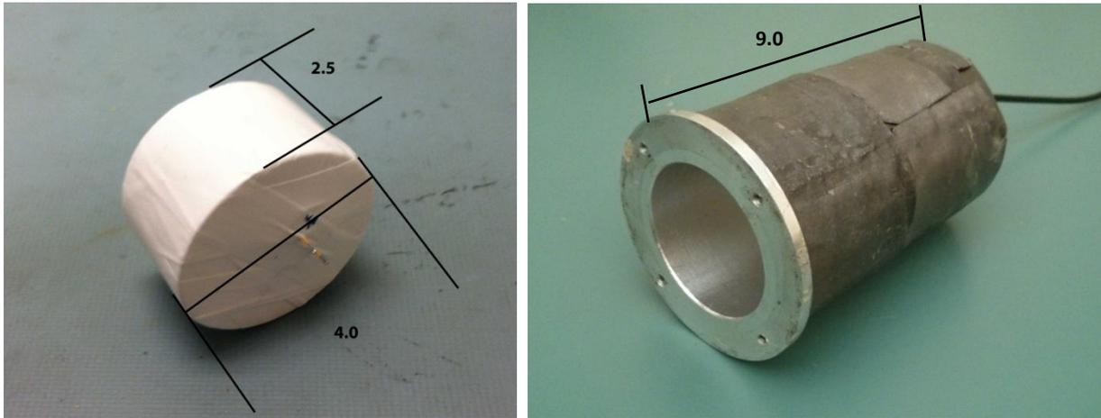
Figure 2. The HAXDT detector is comprised of an APD attached to a plastic scintillator and then wrapped in PTFE tape, shown on the left with dimensions in centimeters. The wrapped assembly is then seated in a lead-shielded aluminum housing to complete the assembled detector, shown on the right with the height indicated in centimeters. The coaxial cable coming out of the detector housing is used to connect the APD to the detector board.
