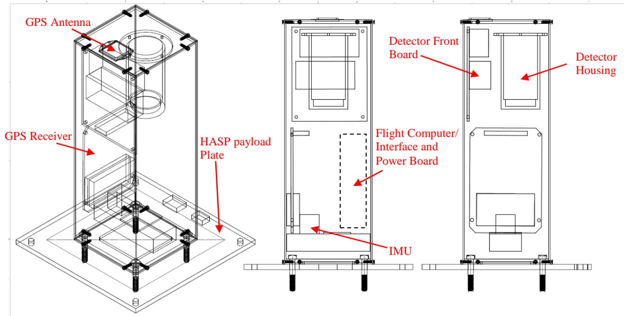
Figure 1. A 3D drawing of the HAXDT structure. The base is 10 cm x 10 cm, while the wall is 30 cm high. All interior hardware is custom mounted as indicated. The detector sits in the cylindrical mount as shown attached to the interior of the upper plate. The dimensions conform to a 3-U CubeSat design and allows for easy reconfiguration of the interior components.
