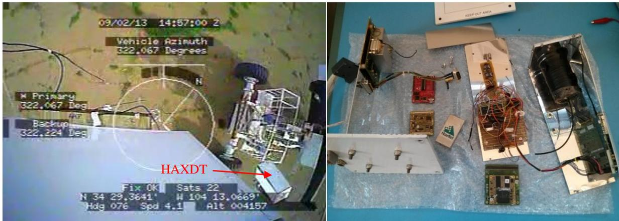
Figure 3. The HAXDT payload falling to the ground after striking the mobile launch vehicle's crane arm (left); the remains of the payload after recovery (right). Note the side panel still loosely attached to the payload plate, which remained attached to the gondola for the full flight.
