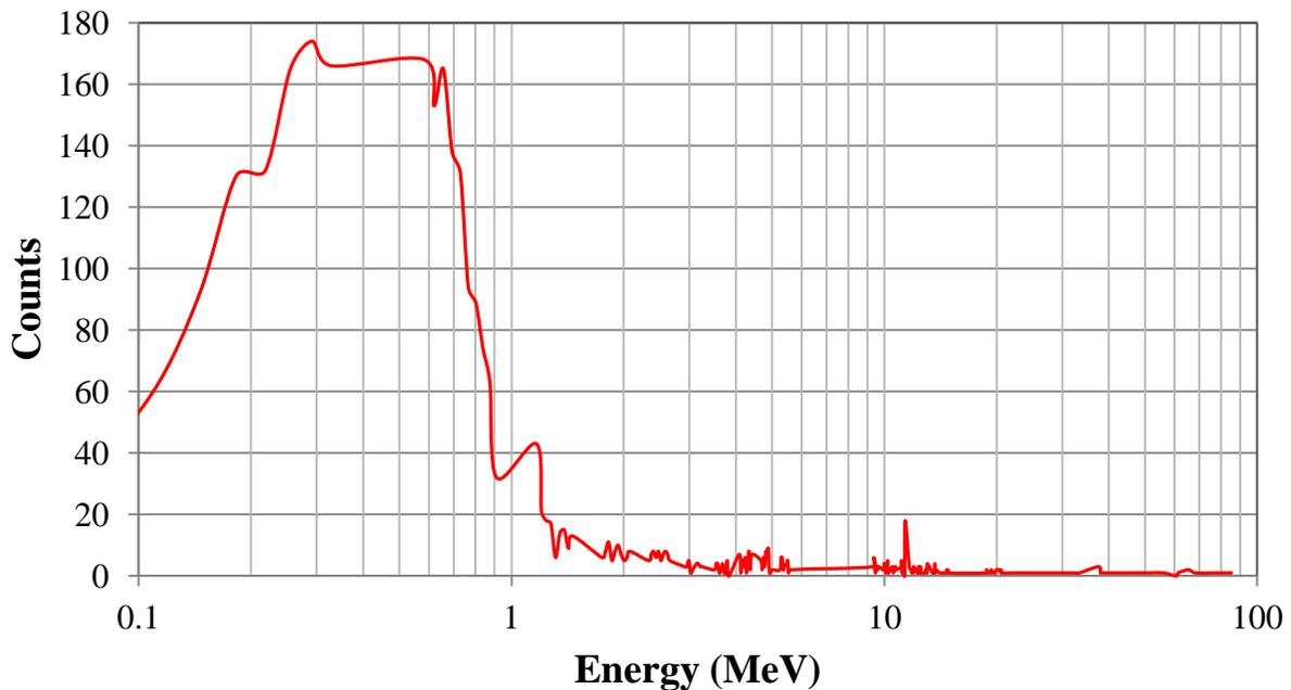
Figure 4. A plot of the photon energy spectrum from a portion of the thermal/vacuum test. Detected events ranged from just below 100 keV to 85 MeV.
