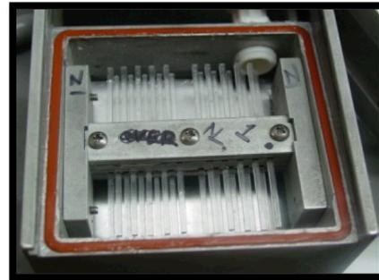
Figure 2: Sampling chamber with 40 silicon covered rods
