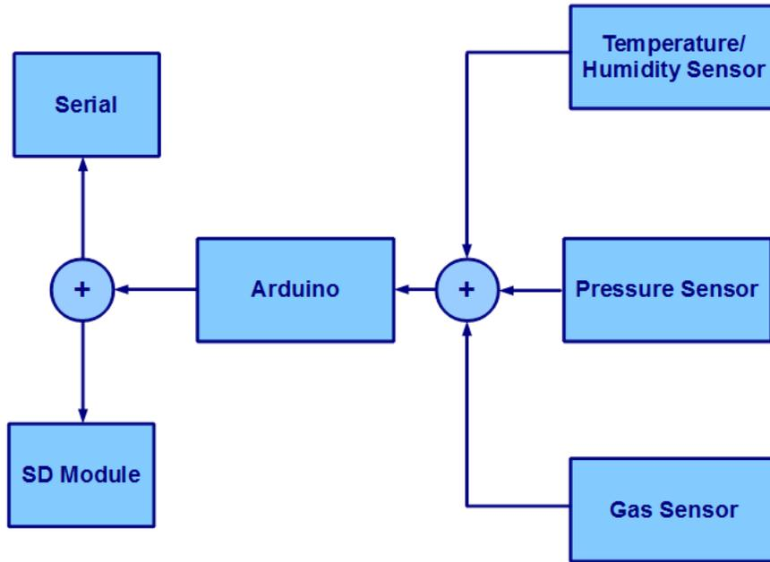
Figure 3. Block diagram showing the payload components that will be used to collect the necessary data for this experiment.
