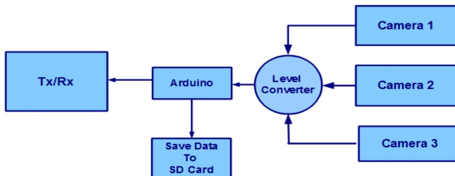
Figure 4. Block diagram showing the payload components that will be used to capture, store, and transmit the images.
