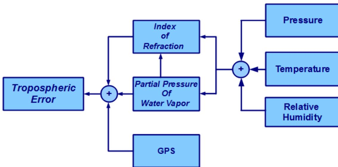
Figure 2. Block diagram showing the payload components that will be used to collect the necessary data for this experiment.
