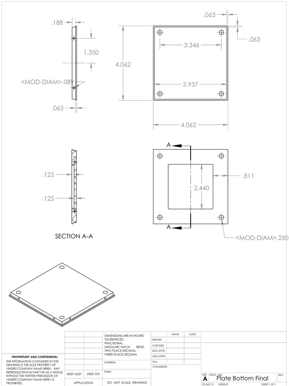
**Figure 12.** Mechanical drawing of bottom plate of 2.5-U and 3-U HAXDT structure with dimensions in inches.
