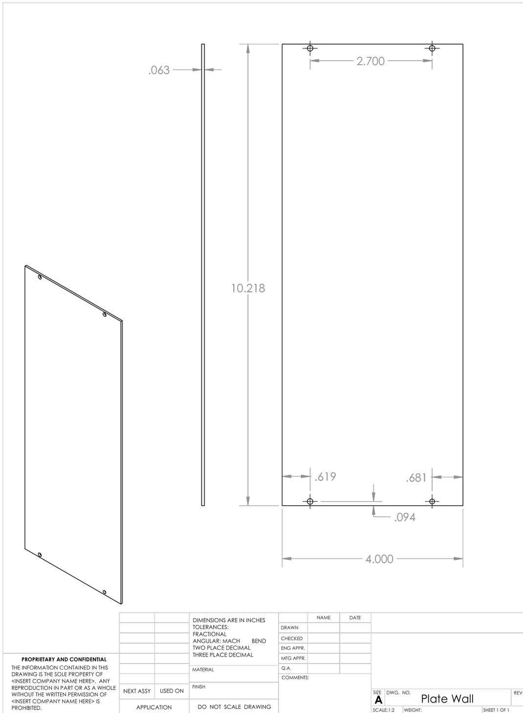
**Figure 13.** Mechanical drawing of 2.5-U HAXDT structure enclosing wall with dimensions in inches.
