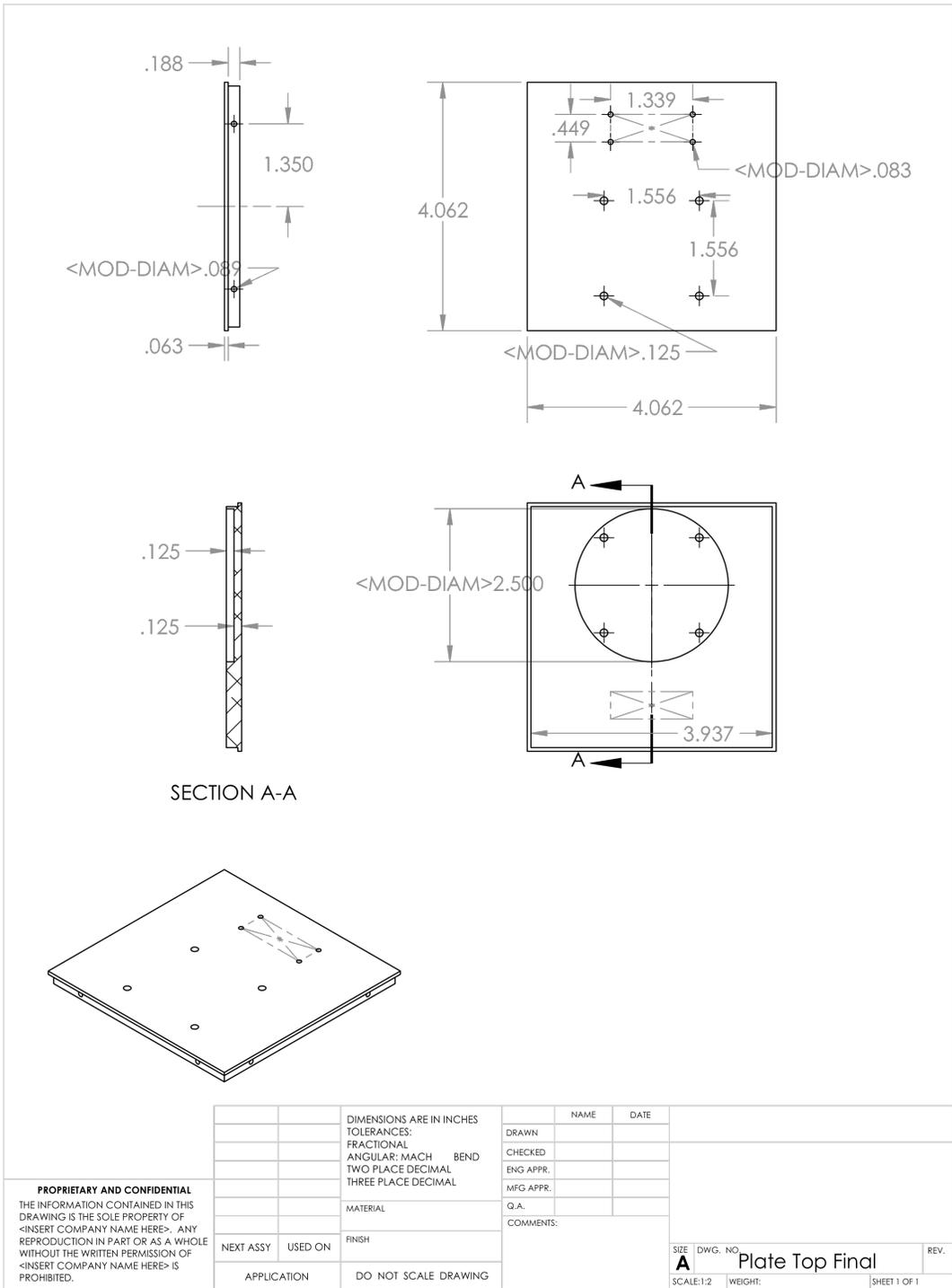
**Figure 17.** Mechanical drawing of top plate of 2.5-U HAXDT structure with dimensions in inches. This plate will be altered to accommodate two detector assemblies.
