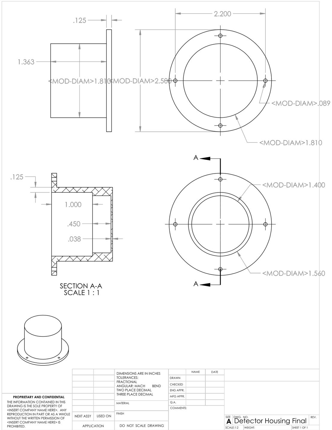
**Figure 2.** Mechanical drawing of detector housing with dimensions in inches. This housing attaches to the top plate of the HAXDT structure (Figure 17).
