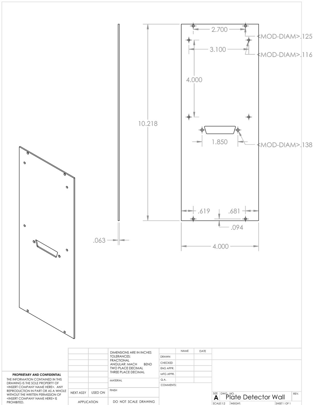
**Figure 15.** Mechanical drawing of 2.5-U HAXDT detector board mounting wall with dimensions in inches. The hole depicted is for a DB-25 connector for the HASP power, serial, and analog lines.
