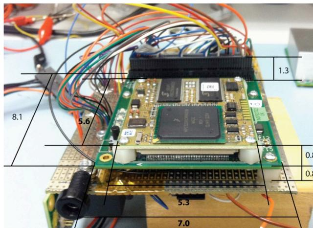
**Figure 8.** Picture of daughterboard (green board) and flight computer (tan board) bundled with the power circuit with dimensions in centimeters.
