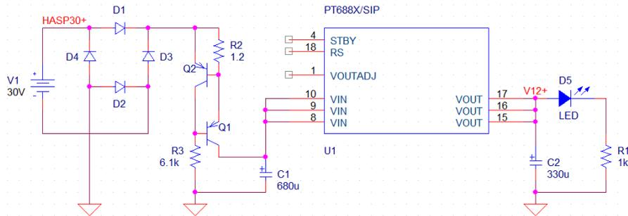
**Figure 10.** Power regulation and protection circuit diagram.
