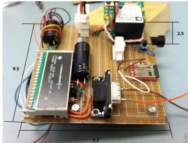
**Figure 7.** Picture of power circuit and Analog Devices IMU with dimensions in centimeters. This board is bundled with the daughterboard and flight computer as seen in Figure 8.
