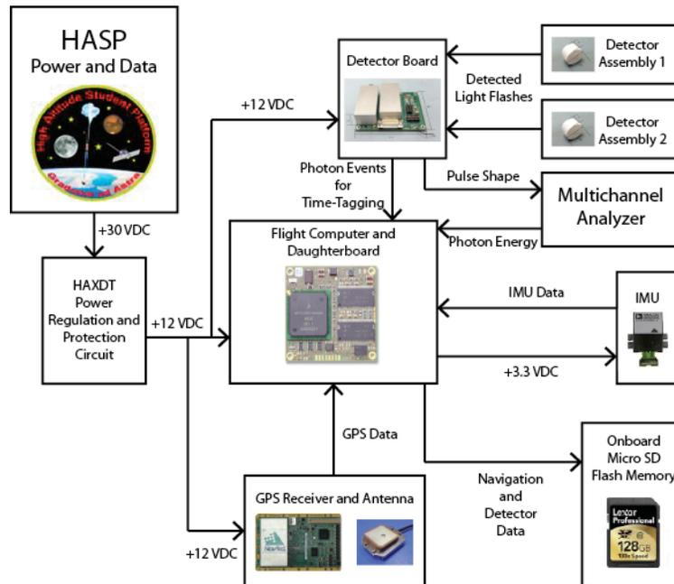
**Figure 1.** High-level HAXDT payload system diagram.
