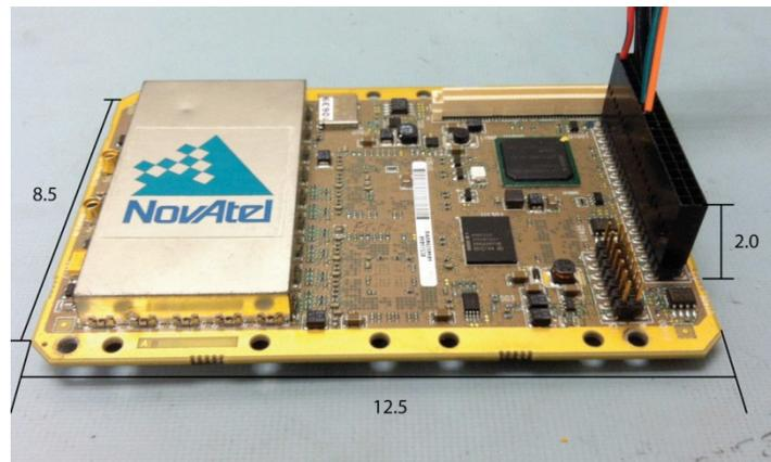
**Figure 5.** Picture of Novatel OEMV-3 GPS receiver and wiring harness with dimensions in centimeters.
