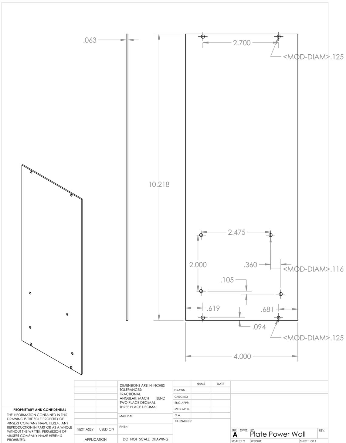
**Figure 16.** Mechanical drawing of 2.5-U HAXDT flight computer/IMU/power circuit bundle mounting wall with dimensions in inches.
