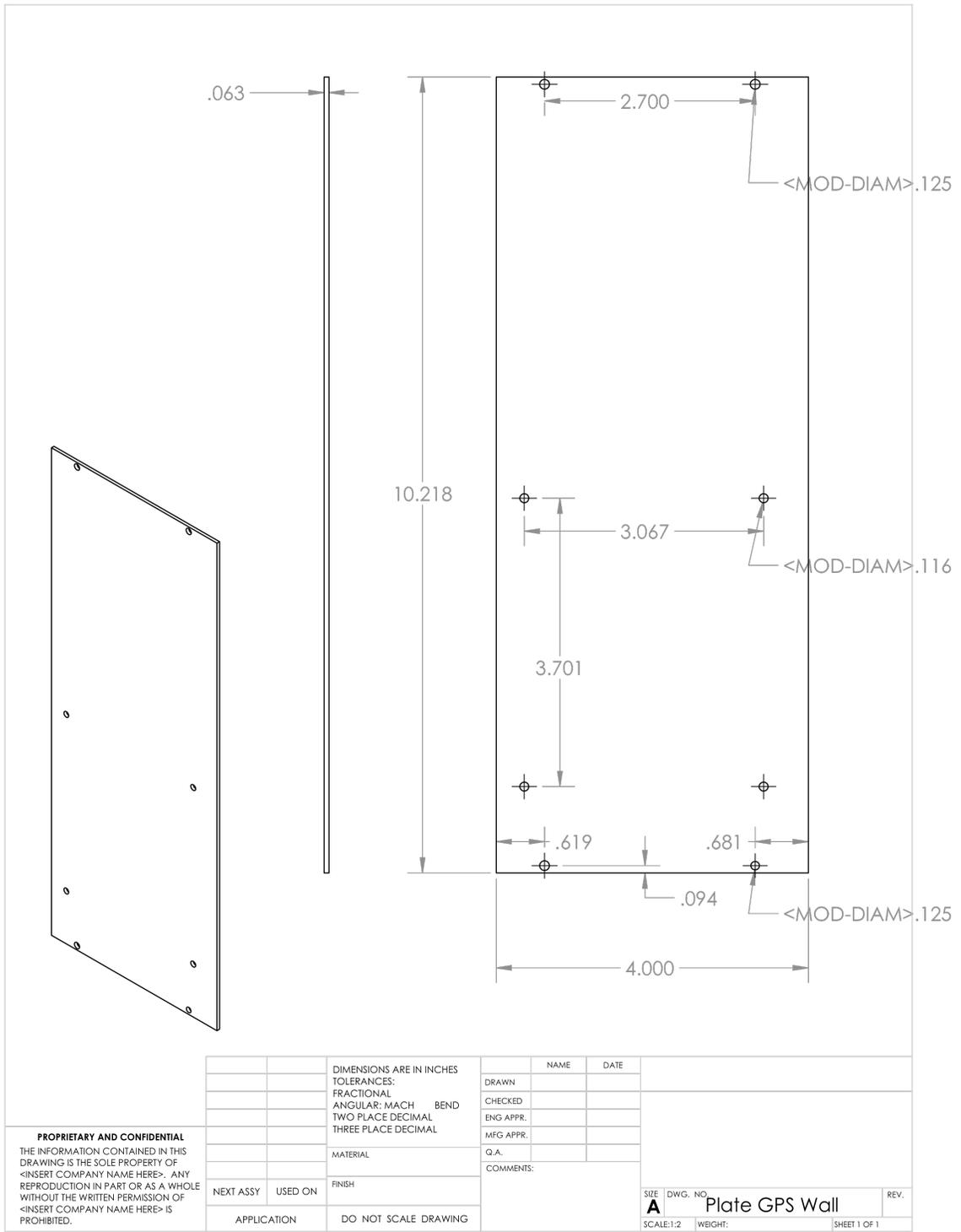
**Figure 14.** Mechanical drawing of 2.5-U HAXDT GPS mounting wall with dimensions in inches.
