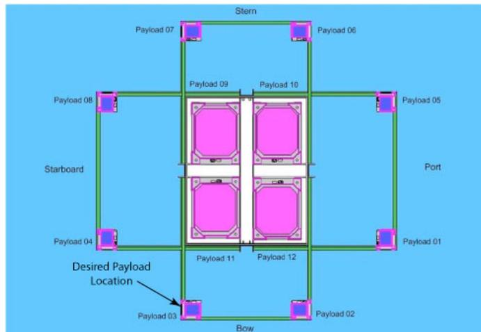
**Figure 19.** Desired payload location on the HASP gondola. Payload orientation does not depend on payload location.
