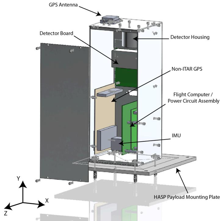
**Figure 11.** 3-D rendering of a 2.5-U HAXDT configuration. This configuration successfully flew on the 2012 HASP mission.
