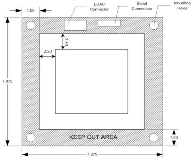
**Figure 18.** Anticipated 3-U HAXDT footprint on the HASP mounting plate. Note that the dimensions of the footprint are 2.50cm (not inches) from the Keep Out Area.
