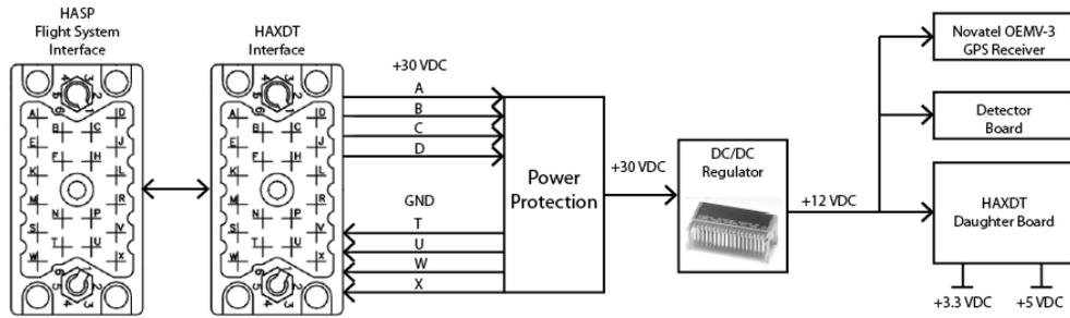
**Figure 9.** Schematic of HASP EDAC516 connector interface with the HAXDT payload power system.
