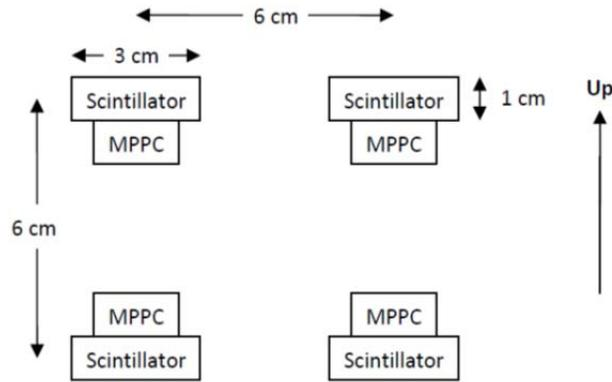
Figure 2. Detector Module - scintillator layout
