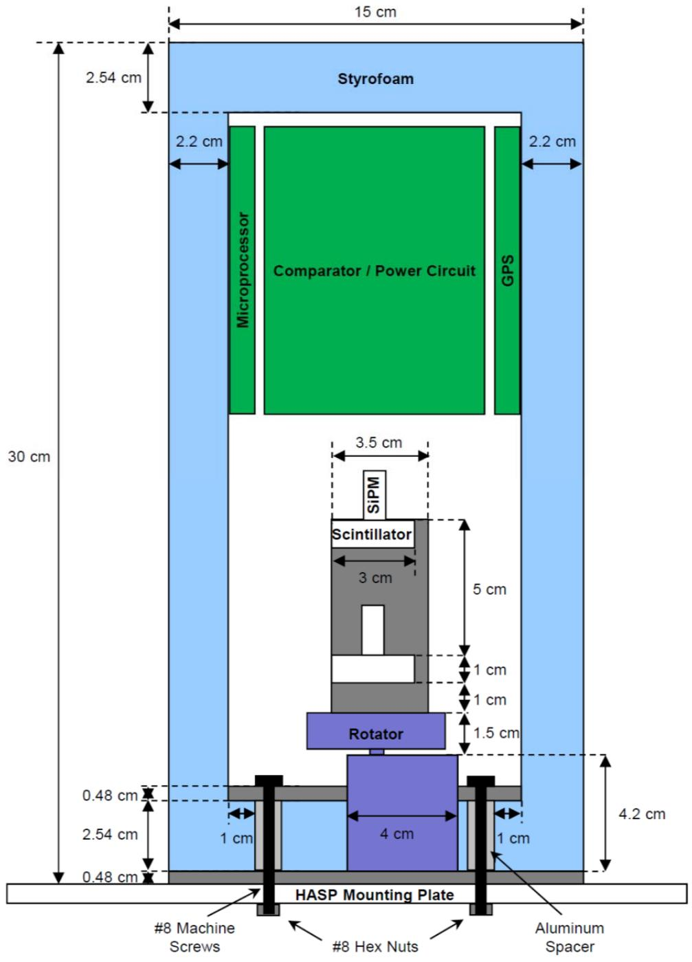
Figure 6. Side cut view of payload
