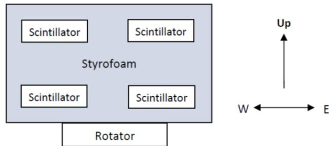
Figure 3. Detector Module with a rotator for position adjustment
