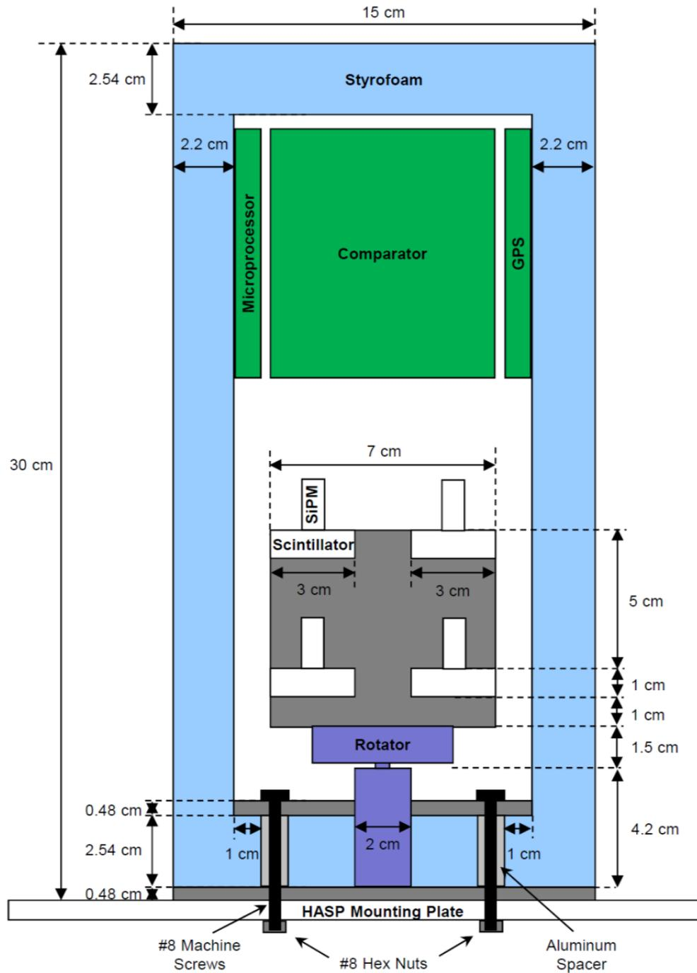
Figure 5. Front cut view of payload
