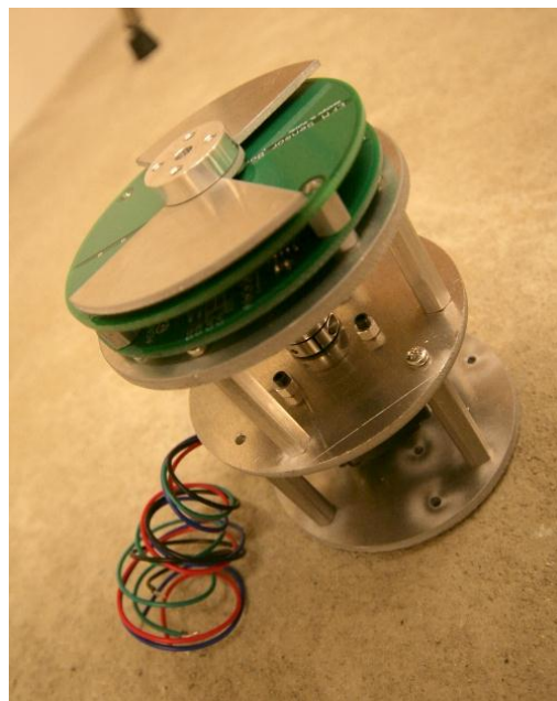
Figure 2: Completed mechanical structure of the EFM supporting both the analog and sensor boards. Wires at bottom left are from stepper motor.
