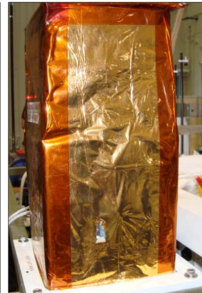
Fig.8c Thermal blanket (golden color) on Payload body
