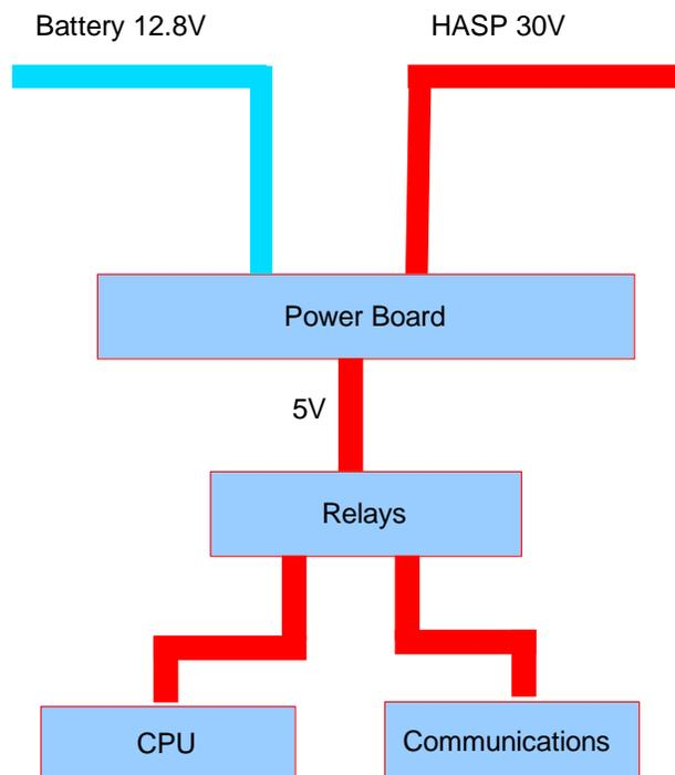
With this method, there is no possibility of the CPU and communications systems being active at the same time.
