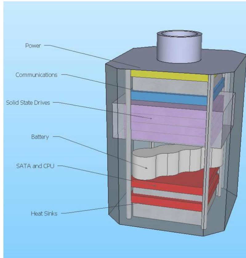
The electrical connections will be wired up to the top of the payload. The hard drives will be enclosed in their own aluminum enclosure as needed. This will help spread out heat generated and allow for 1 relay switch to turn on/off hard drive heat if needed. The batteries will be placed in between the board stack and the hard drives.
