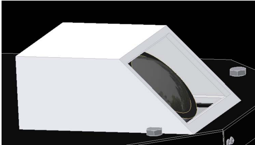
Figure 8 - Antenna enclosure made of foam core and Mylar window for undistorted signal.
