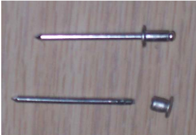
Figure 12: Pop-rivet before and after use.
