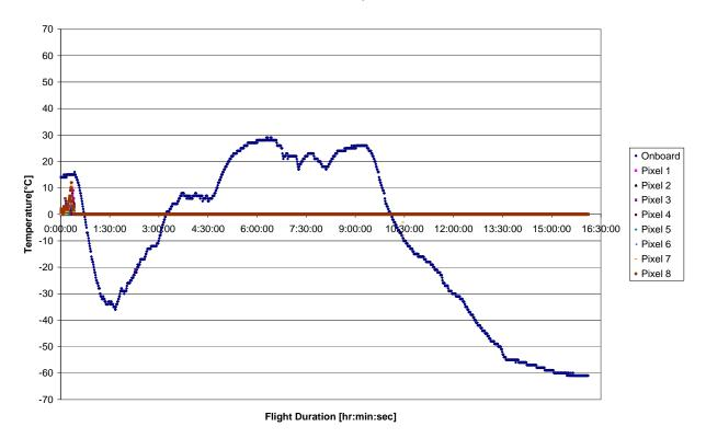
Figure 10. Sensor 4 (~90° arc position) temperature data.
