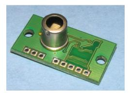
Figure 3. Devantech 8x1 thermopile array.
