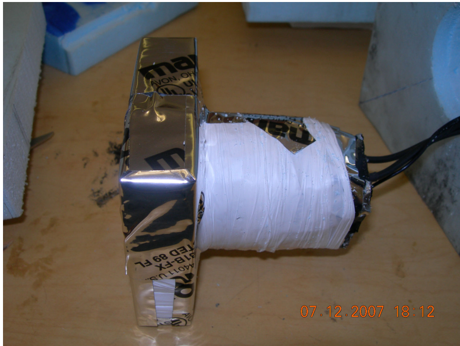
Figure 3: Single Light Tight Detector Assembly
