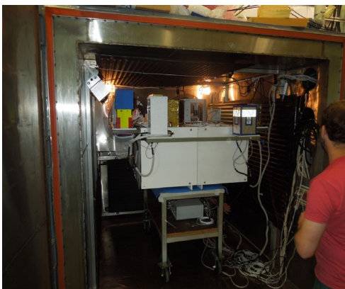
Figure 8: HASP and student payloads in the CSBF BEMCO chamber in preparation for thermal / vacuum testing.
