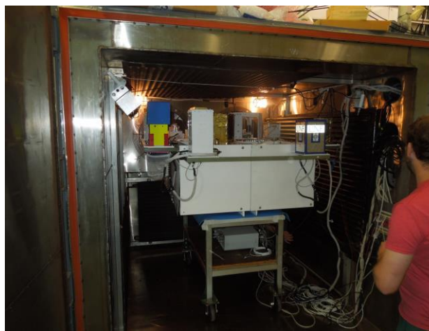
Figure 8: HASP and student payloads in the CSBF BEMCO chamber in preparation for thermal / vacuum testing.
