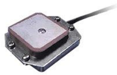
Figure 6. Picture of San Jose Technology, Inc. SA60 GPS antenna, which attaches to the outside of the top plate as seen in Figure 12.
