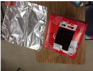
2. Cut a piece of aluminum foil to fit over the cut in the top of the box you just made. The foil needs to completely cover the hole and there should be no tears in the aluminum foil. Tape the foil in place so that it will not come off the end of the box.
