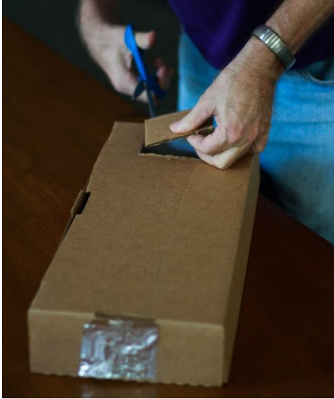
5. Cut a window close to the screen to be able to view the image. Tape the box closed.
