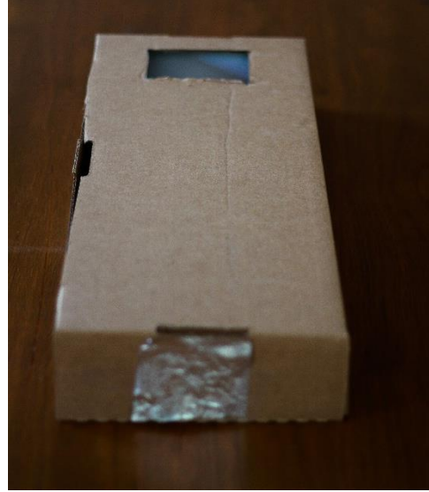
6. The box is ready for use. You can see the screen through the window. The aluminum foil with the pinhole will point at the sun.
