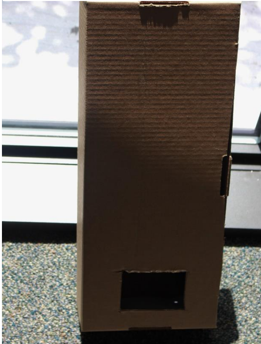
7. Viewer with pinhole pointed at the sun. You can see the bright image of the sun through the window.
