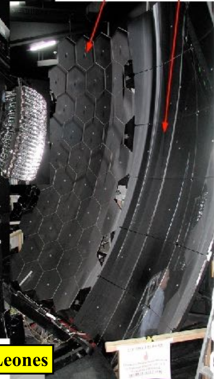
two types of mirrors (for testing) glass aluminum
