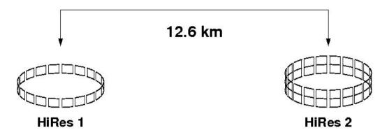
The HiRes fluorescent detector in Utah consisted of two telescopes with slightly different field of view. One of them looks at elevations of 3 to 17 degrees and the other one from 3 to 31 degrees. They can also work in coincidence.
