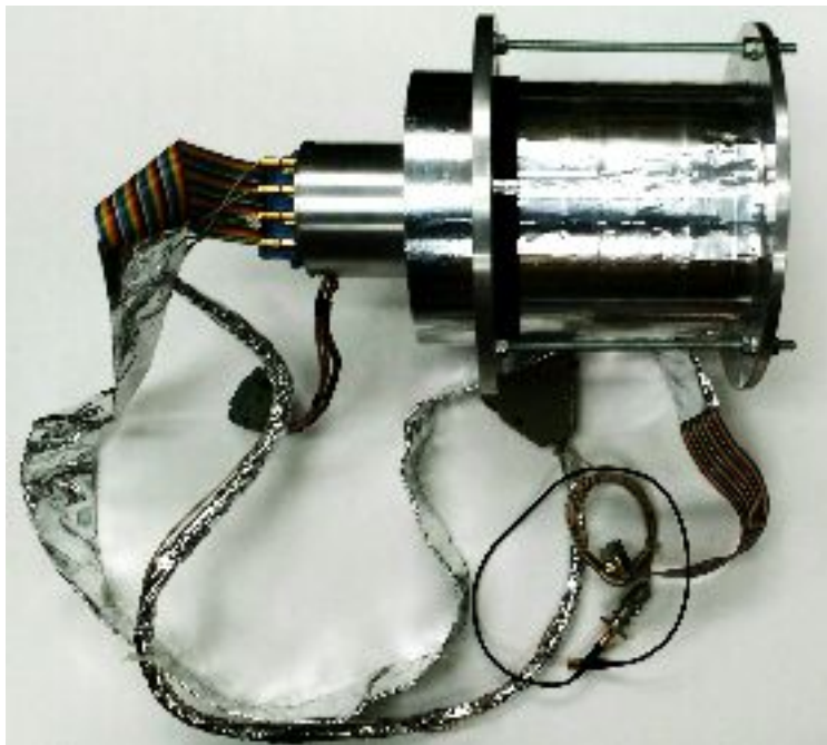
Fig. 11 - The CACT \mu S CdTe detection cylinder and cabling are shown here.
