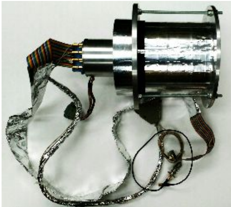
Fig. 8 - The CACT \mu S CdTe detection cylinder and cabling are shown here.
