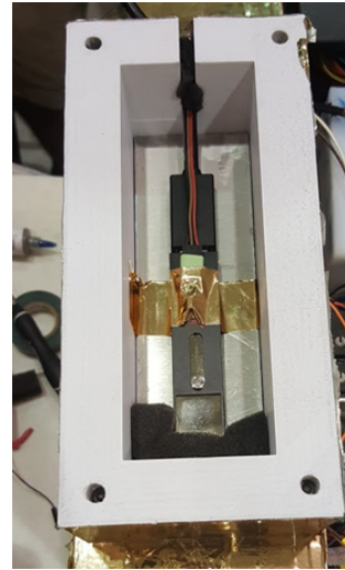
FIG. 7. Picture of the MiniPIX mounted in the case and heat sink assembly on SORA 1.0.
