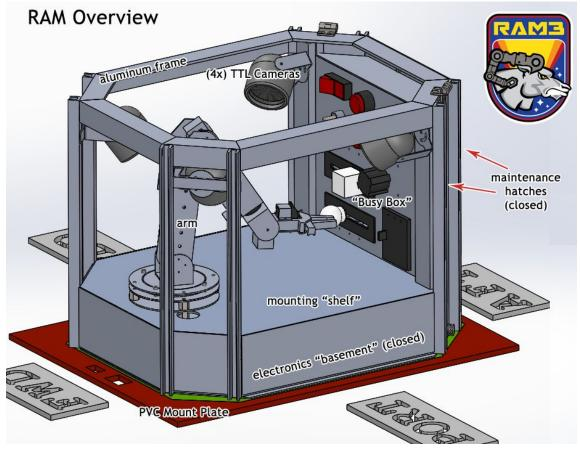
Please note that in all renders we have omitted the cradle and the arm-mounted PixyCam; we need more testing to determine their orientation, balance, and placement.
