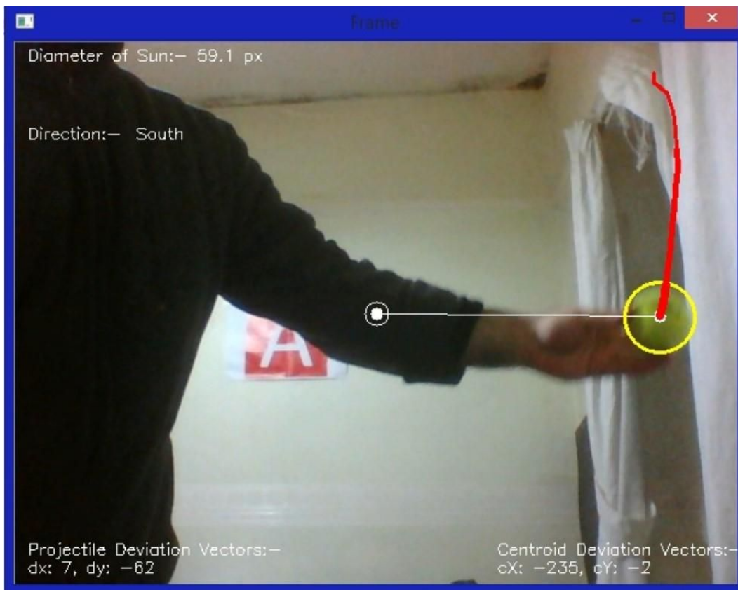
Figure 4.3.2.1. – Visual tracking algorithm tested on a tennis ball prototype.
