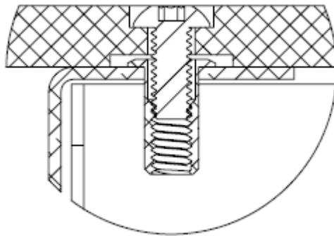
*Figure 7: Fastener Cross-Section*
