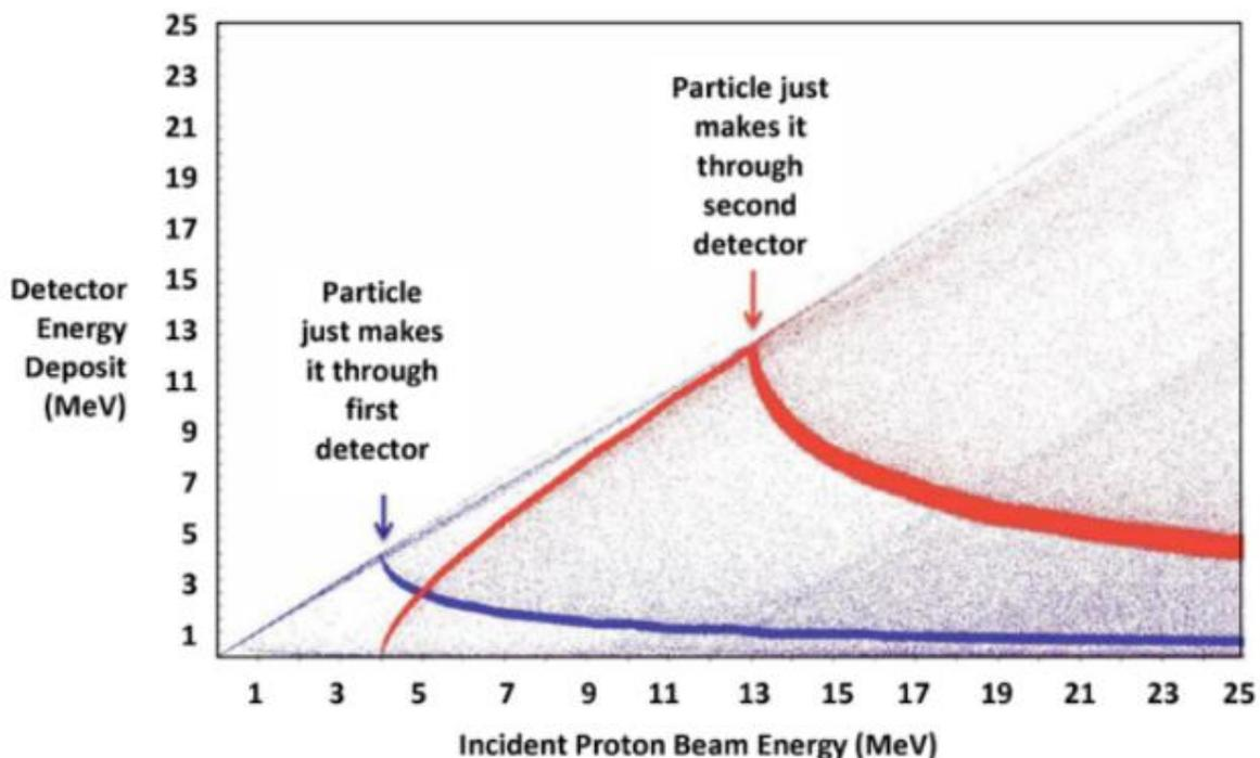
Figure 1: Simulation Plot of Cosmic Ray Signals in a Silicon Diode Telescope [1]
