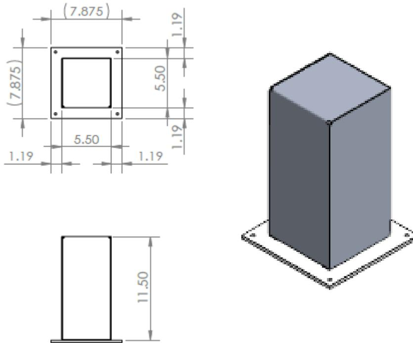
*Figure 5: Proposed Payload Dimensions*
