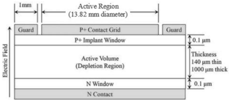
Figure 10: Schematic cross section of the silicon detector
