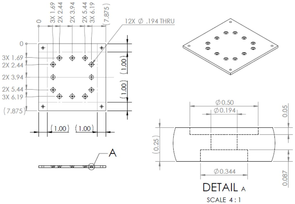
Figure 8: Dimensioned Drawing of Modified Payload Mounting Plate
