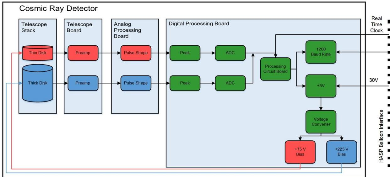
Figure 2: Functional Block Diagram of Cosmic Ray Detector
