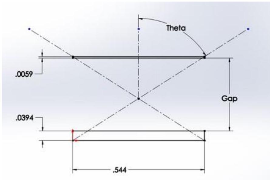
Figure 9: Viewing Angle of Detector
