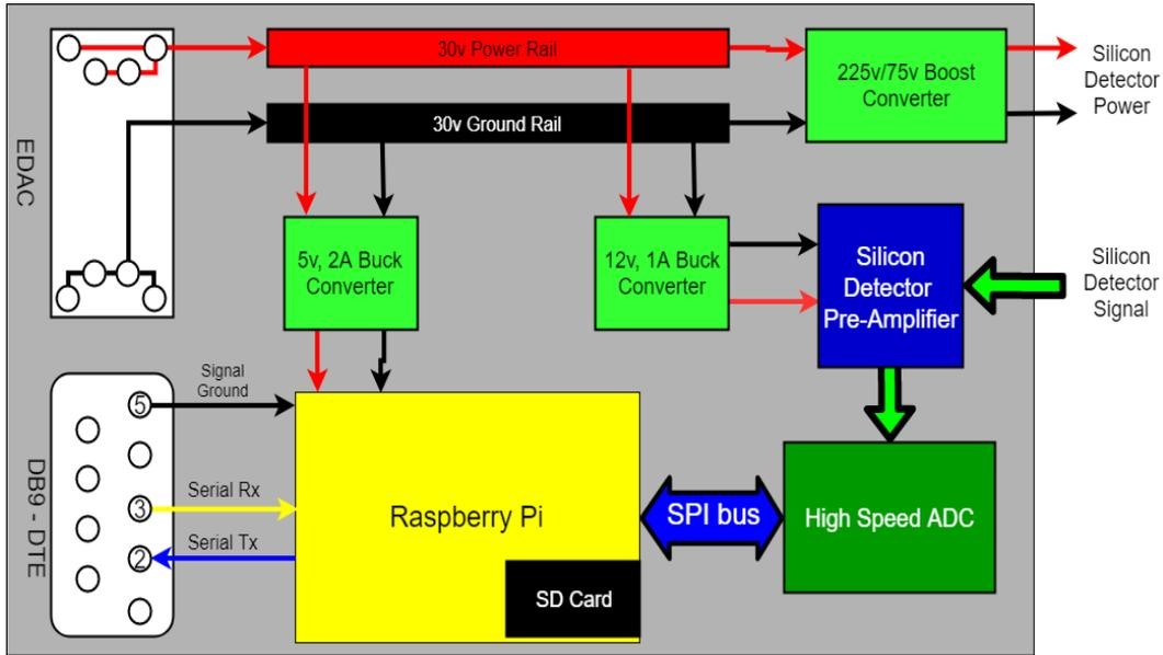
Figure 3: Wiring Block Diagram
