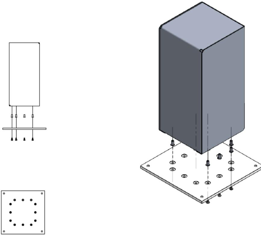
*Figure 6: Payload Mounting Plate Interface*
