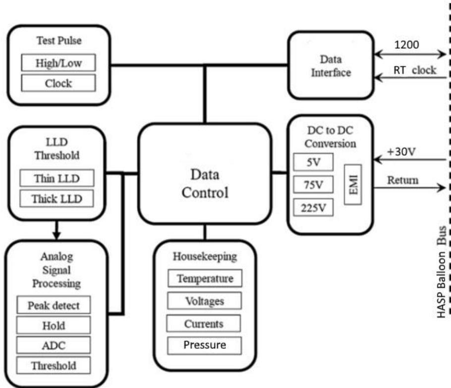
Figure 14: Functional Block Diagram of Flight System
