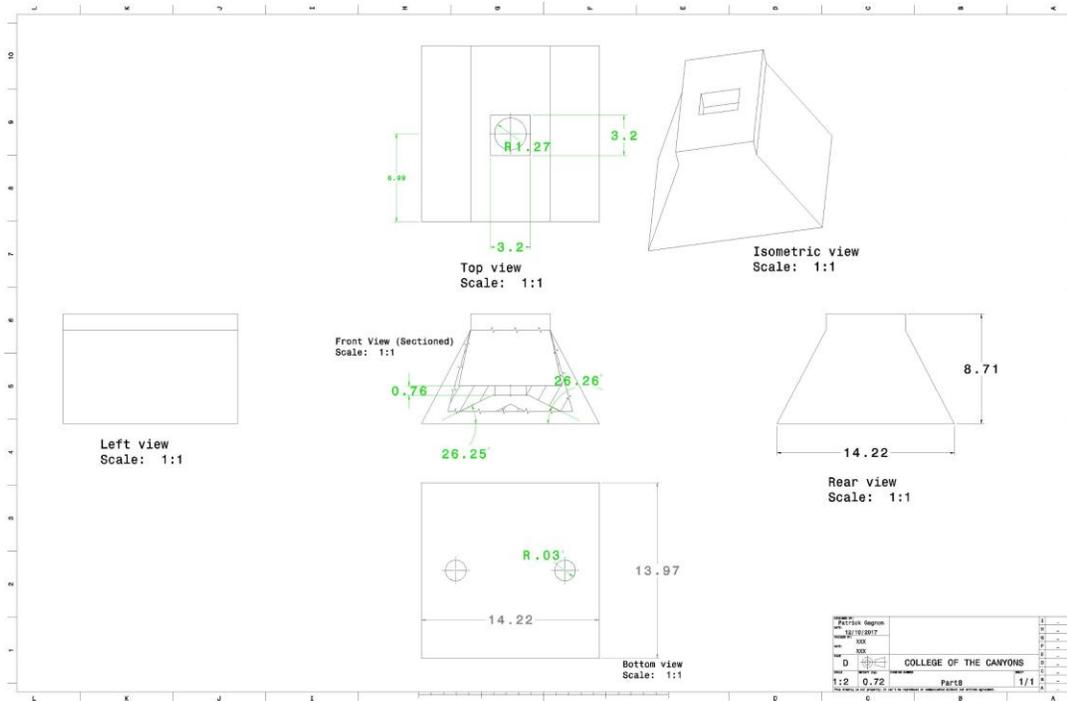
Figure 7.2.2A - Intake Drawing
