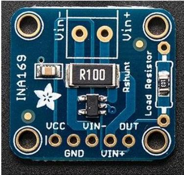
Fig 2.3.2D – Current Sensor
