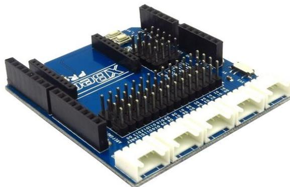
Fig 2.5.1A – Arduino Sensor Shield
