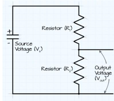
Fig 2.3.2E – Voltage Sensor
