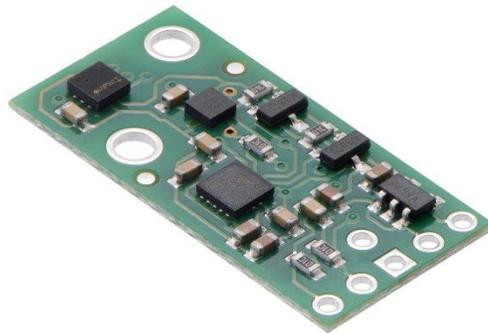
Fig 2.5.6A – Gyroscope, Altimeter, and accelerometer
