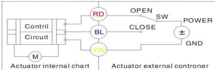
When **RD** & SW connected, the valve opens, the actuator automatically powers off after it is in place, the valve remains fully open position.
