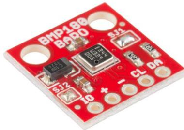
Fig 2.5.3A – Pressure sensor
