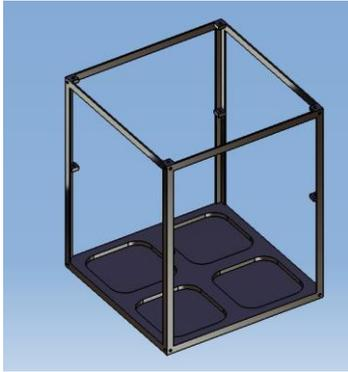
material for College of the Canyons for its ease of machining, strength, weight, and previous successes. We have familiarity with the stress/strain and thermal capabilities of the aluminum 2024 from previous HASP missions and know it will provide the necessary support to endure the 10g vertical and 5g horizontal forces while protecting encased components.
