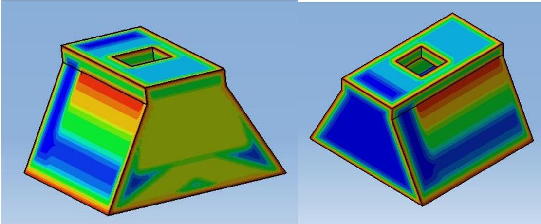
Figure 2.2.7 - Wall thickness Analysis on nylon intake
