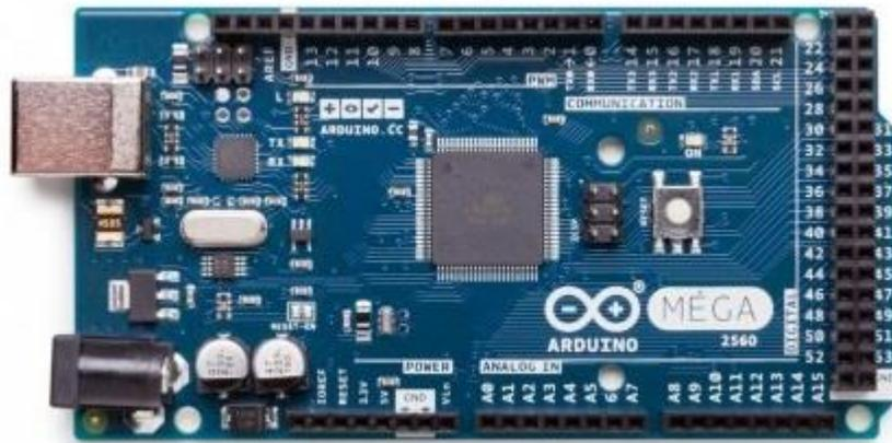
Fig 2.4.1A – Arduino Mega
