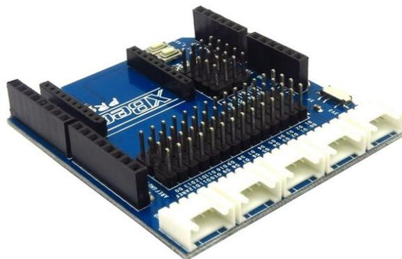
Fig 2.5.1A – Arduino Sensor Shield
