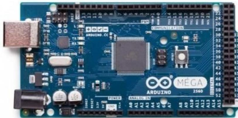
Fig 2.4.1A – Arduino Mega
