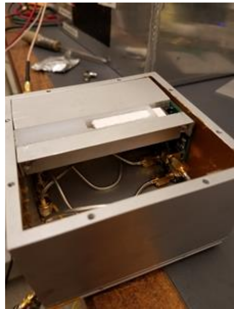
Figure 2: A single channel engineering prototype of CITIES.
