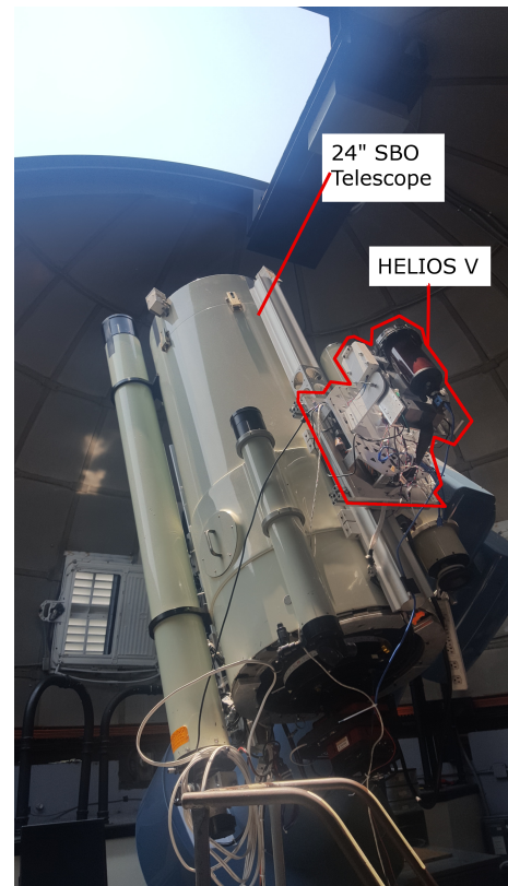
Figure 23: HELIOS V attached to the SBO telescope
