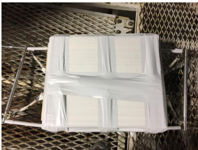
Figure 3. The flight ladder payload attachment system. Two steel cables secure the payload to the fifth rung (left) and two steel cables secure the payload to a temporary rung (right). PVC reinforces the steel cables of the flight ladder where four steel cable loops attach the sides of the box.
