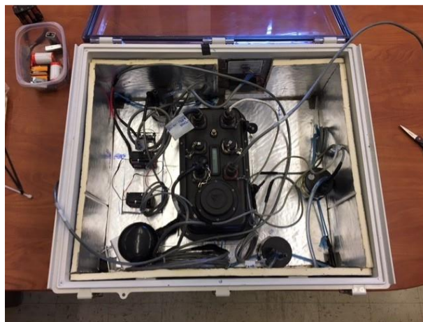
Figure 2. The internal workings of the flight ladder payload. Three InfraBSU infrasound microphones are enclosed in cases with a white PVC body and a securely fit black top. The ADXL accelerometer is mounted to the side of the box. The Trimble RefTek130S-01 logger sits in the middle, with its GPS in the bottom left corner. The power system sits to the left of the RefTek.
